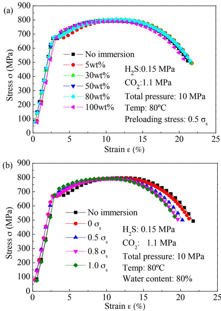
**Figure 6.** Dependence of stress–strain curve of L80 steel on: (a) water content; and (b) preloading stress after immersion in the test medium for 720 h.
