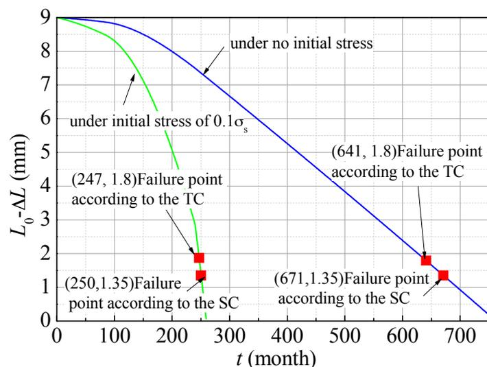
**Figure 12.** Variation of residual wall thickness of L80 steel with service time under different initial stress: 0 and  $0.1 \sigma_s$ , respectively.
