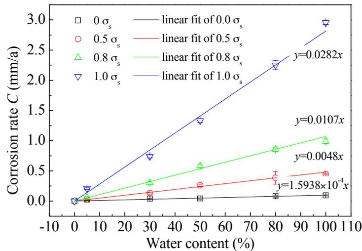
**Figure 8.** Corrosion rates of L80 steel and their fittings as a function of water content under different preloading stress.
