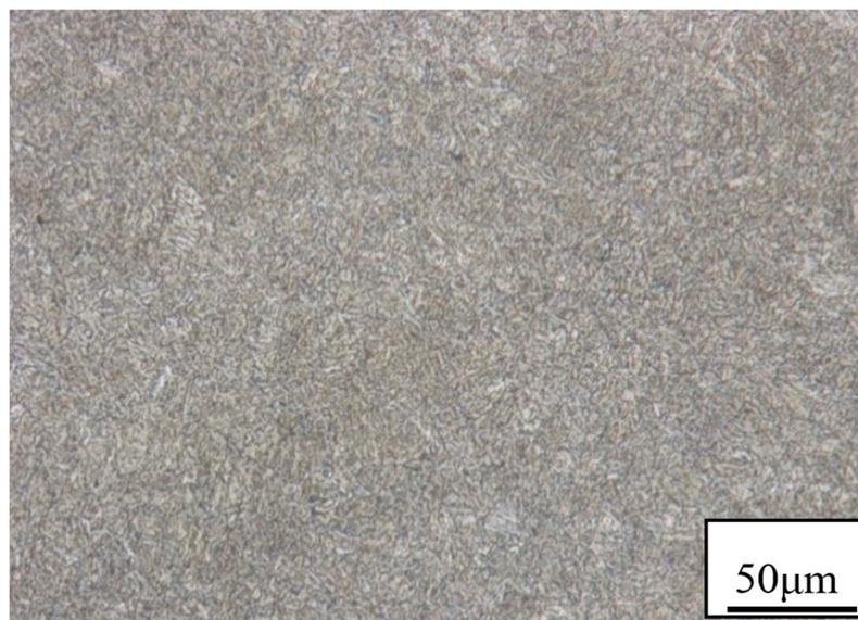
Figure 1. Microstructure of L80 steel.
