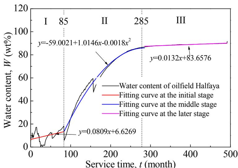
**Figure 2.** Dependence of water content of oilfield Halfaya on service time.
