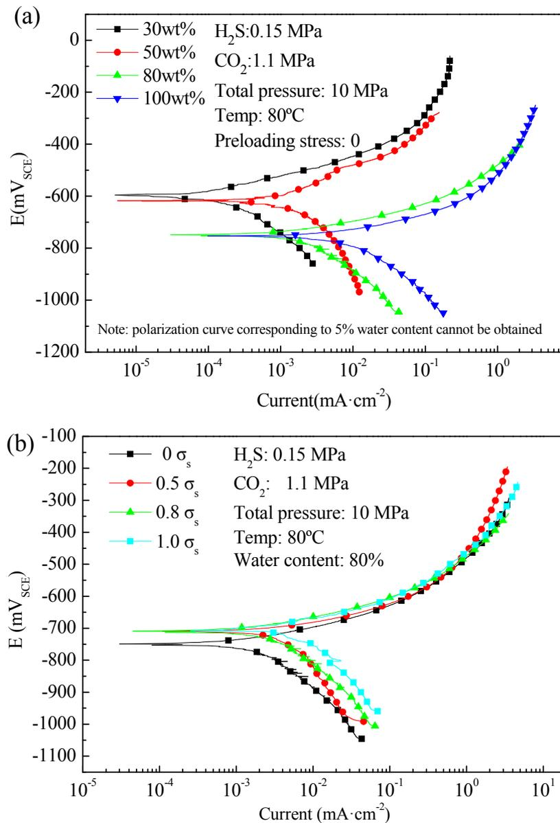
Figure 4. Potentiodynamic polarization curves of L80 steel measured under different: (a) water contents; and (b) preloading stresses.
