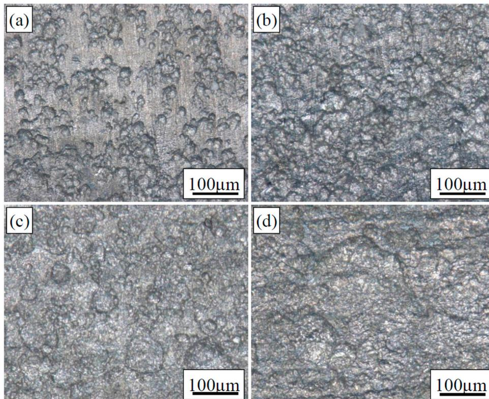
**Figure 5.** Corrosion morphology of L80 steel after immersed in the medium of 80 wt % water content for under preloading stresses of: (a)  $0 \sigma_s$ ; (b)  $0.5 \sigma_s$ ; (c)  $0.8 \sigma_s$ ; and (d)  $1.0 \sigma_s$ .
