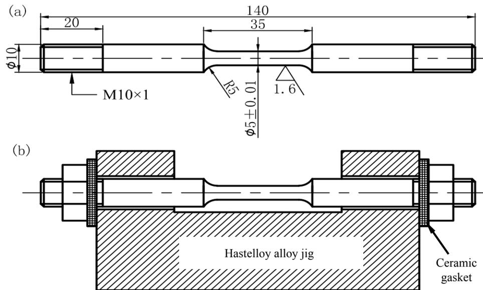
**Figure 3.** Sizes of (a) the specimen and (b) the assembling jig used for preloading.
