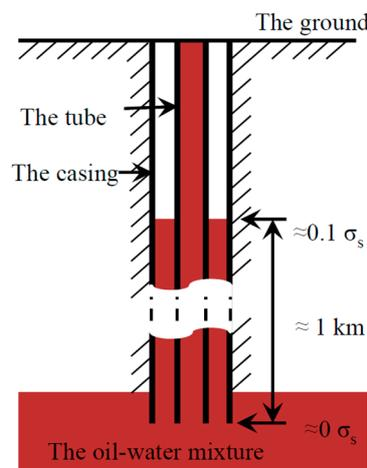
Figure 11. The initial stresses that different parts of the downhole tube or casing suffer.
