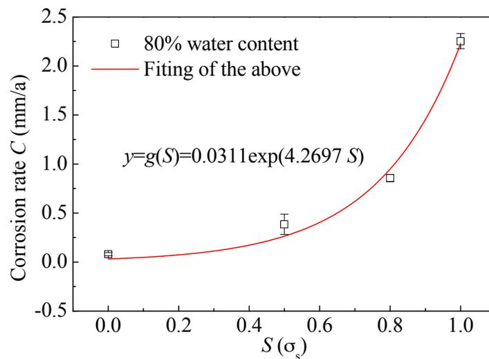
**Figure 9.** Dependence of corrosion rate of L80 steel at 80% water content on preloading stress.
