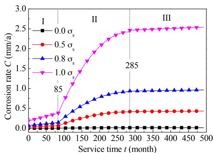
**Figure 10.** Corrosion rates of L80 steel as a function of service time under different preloading stress.
