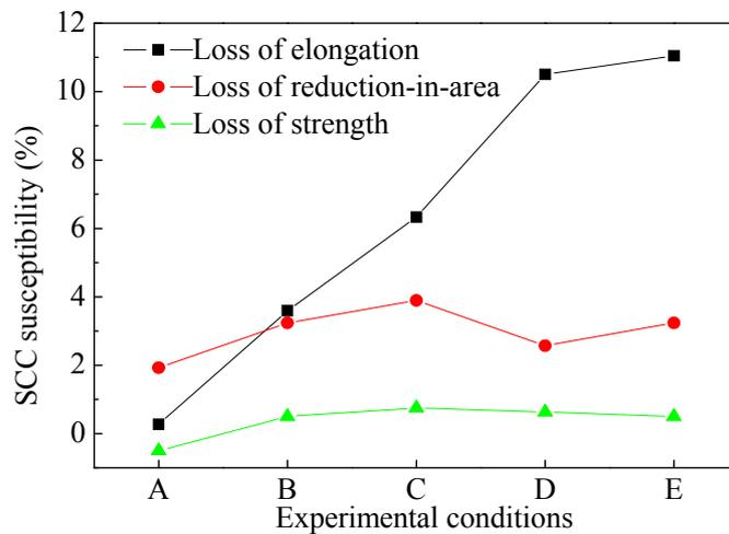
**Figure 7.** Variation of SCC susceptibility of L80 steel after immersion for 720 h with water content and preloading stress (A: 5 wt %,  $0 \sigma_s$ ; B: 80 wt %,  $0 \sigma_s$ ; C: 80 wt %,  $0.5 \sigma_s$ ; D: 80 wt %,  $0.8 \sigma_s$ ; and E: 80 wt %,  $1.0 \sigma_s$ ).
