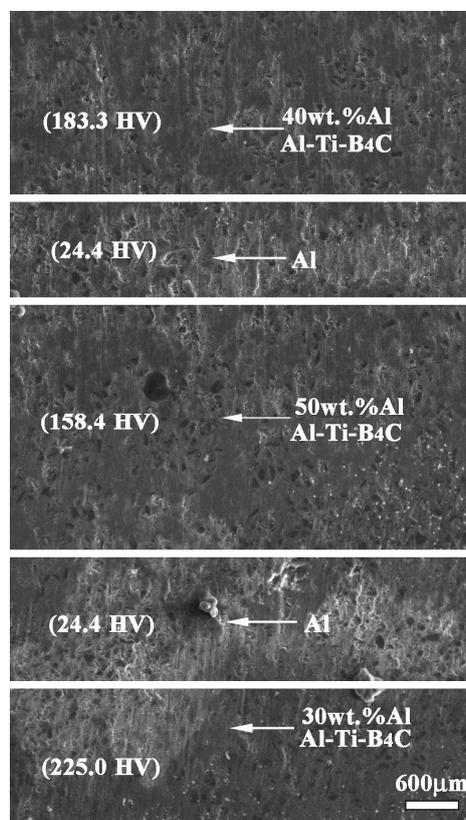
**Figure 3.** Metallography and microhardness of bionic layered composite.
