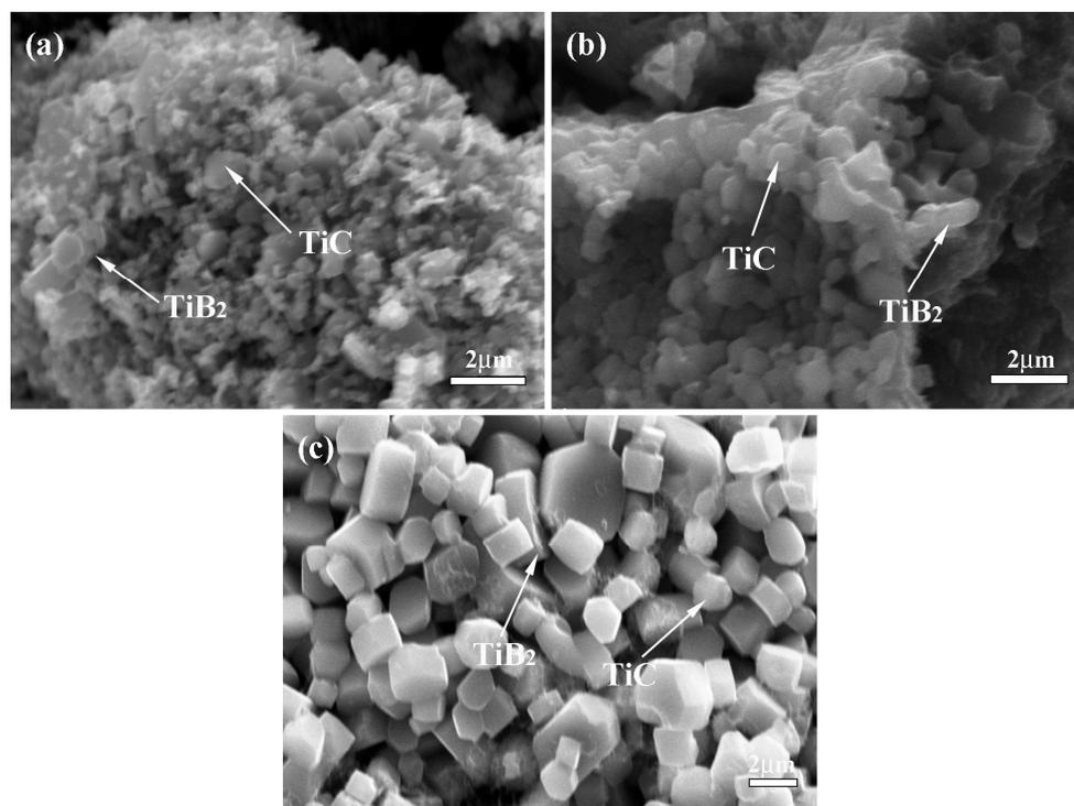
**Figure 4.** Fracture morphology of bionic layered composite (a) outer layer (b) middle layer (c) inner layer.
