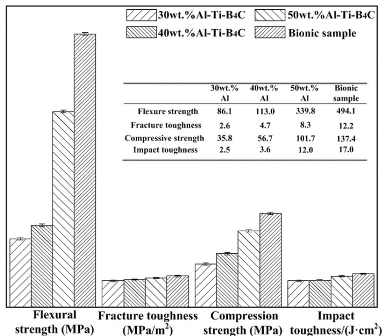
**Figure 6.** Flexural strength, fracture toughness, compression strength and impact toughness values of 30 wt. %–50 wt. % Al-Ti-B<sub>4</sub>C composite and bionic layered composite.
