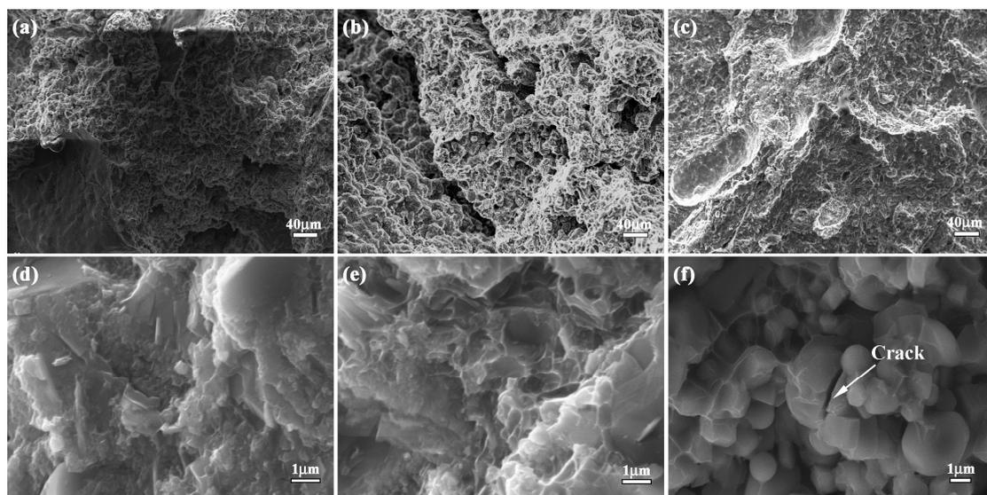
**Figure 10.** Impact appearance of bionic layered composite (a) outer layer (b) middle layer (c) inner layer (d) magnified microstructure of (a); (e) magnified microstructure of (b); and (f) magnified microstructure of (c).
