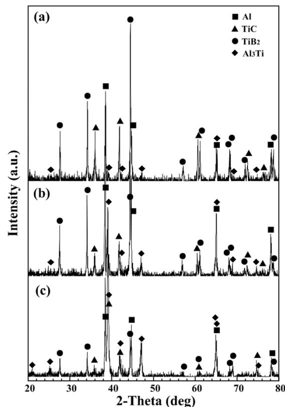
**Figure 5.** Phase identification of bionic layered composite (a) outer layer (b) middle layer (c) inner layer.
