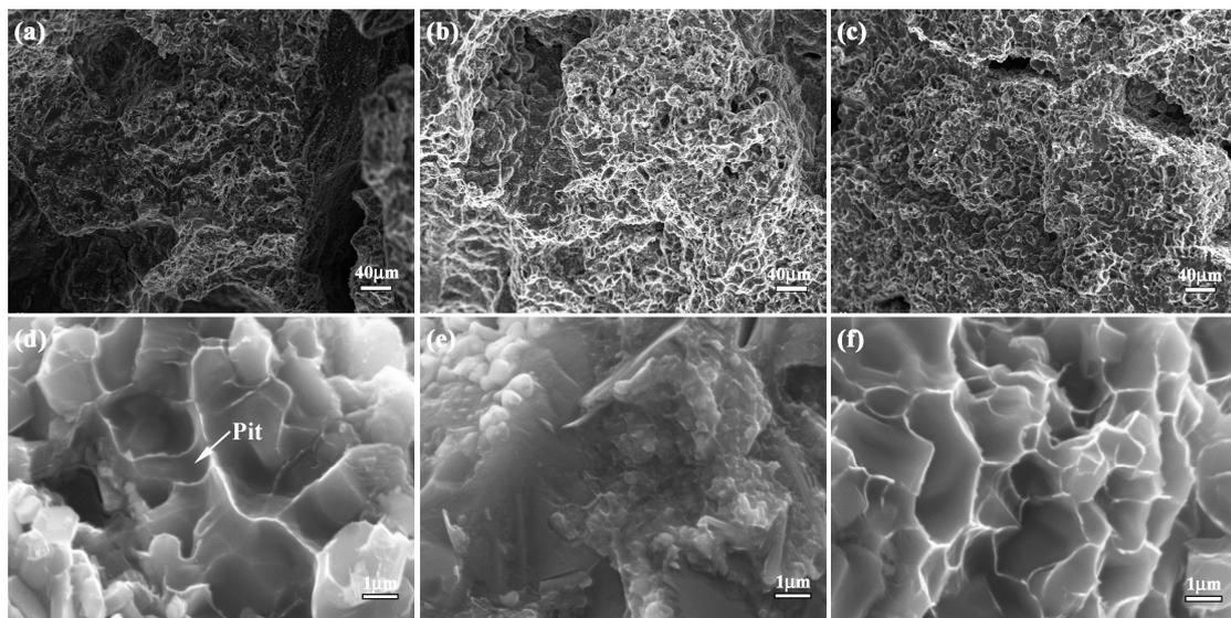
**Figure 7.** Flexural appearance of bionic layered composite (a) outer layer (b) middle layer (c) inner layer (d) magnified microstructure of (a); (e) magnified microstructure of (b); and (f) magnified microstructure of (c).
