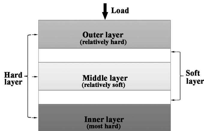
Figure 2. Diagrammatic sketch of bionic coupling impact resistance model.
