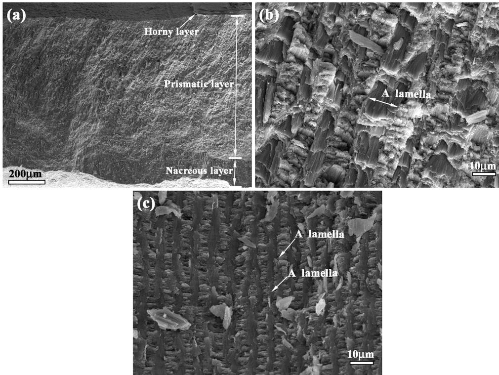
Figure 1. Microstructure of *white clam* shell (a) horny layer (b) prismatic layer and (c) nacreous layer.
