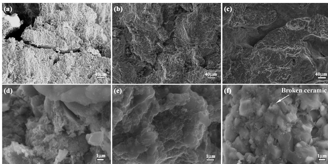
**Figure 9.** Compression appearance of bionic layered composite (a) outer layer (b) middle layer (c) inner layer (d) magnified microstructure of (a); (e) magnified microstructure of (b); and (f) magnified microstructure of (c).
