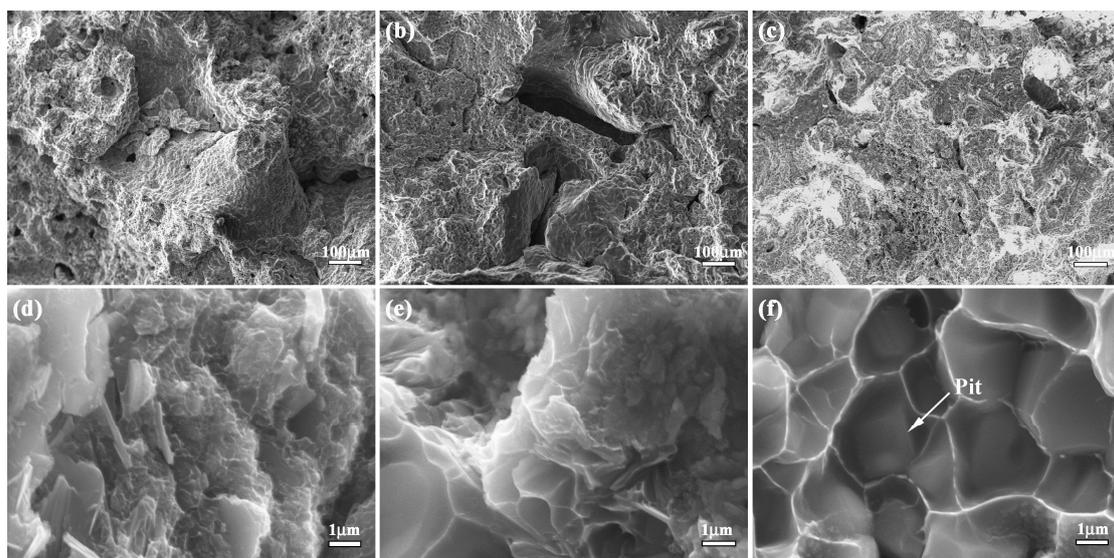
**Figure 8.** Fracture appearance of bionic layered composite (a) outer layer (b) middle layer (c) inner layer (d) magnified microstructure of (a); (e) magnified microstructure of (b); and (f) magnified microstructure of (c).
