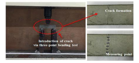
**Figure 2.** View of the three-point bending test for crack introduction, and view of the crack from the lower end of the mortar prism.
