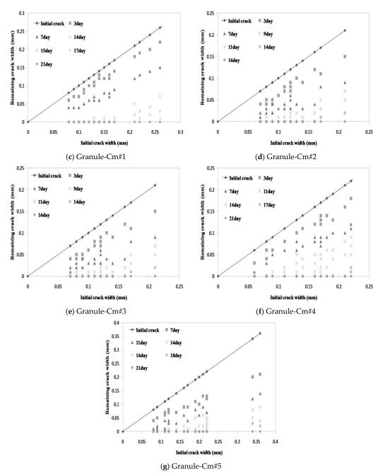
**Figure 5.** Changes in the crack width at each observation day: (**a**) Plain; (**b**) Granule-EA (CSA-based expansive agent); (**c**) Granule-Cm#1; (**d**) Granule-Cm#2; (**e**) Granule-Cm#3; (**f**) Granule-Cm#4; and (**g**) Granule-Cm#5.
