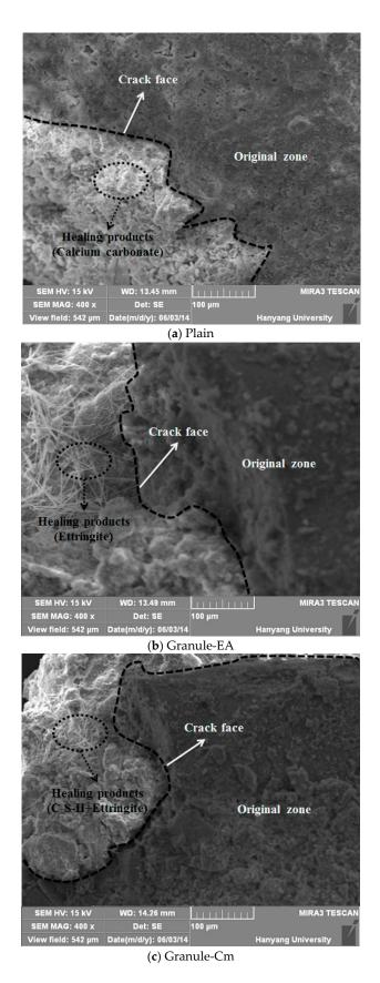
**Figure 11.** SEM micrographs of the healing products that were formed at the crack face (×400): (**a**) Plain; (**b**) Granule-EA; and (**c**) Granule-Cm.
