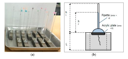
**Figure 4.** Schematic view of the water permeability test. (**a**) Water permeability test being conducted on cracked mortar prism beams; (**b**) longitudinal-cross-sectional view of these specimen under test.
