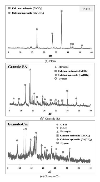
**Figure 10.** XRD pattern of the healing products in the crack face: (**a**) Plain; (**b**) Granule-EA; and (**c**) Granule-Cm.
