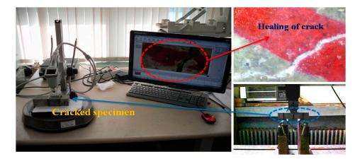
Figure 3. Investigation of crack width with a microscope.
