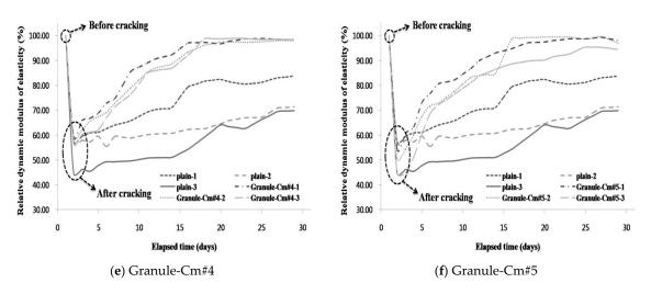
**Figure 7.** Comparison of the relative dynamic modulus of elasticity values of the mixtures: (1: <0.1 mm; 2: 0.1–0.2 mm; 3: >0.2 mm): (a) Granule-EA (CSA-based expansive agent); (b) Granule-Cm#1; (c) Granule-Cm#2; (d) Granule-Cm#3; (e) Granule-Cm#4; and (f) Granule-Cm#5.
