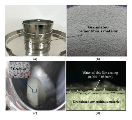
**Figure 1.** (a) Granulating machine; (b) a closer view of the granules obtained from the granulating machine; (c) granules tumbling over one another in the rotating pan where they were dried with hot air before they were sprayed with PVA solution; and (d) the PVA coating of the granules.
