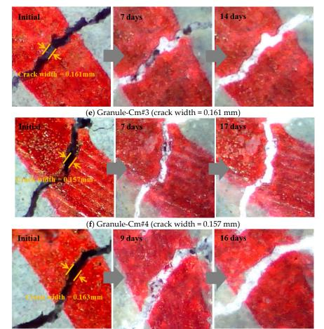
(g) Granule-Cm#5 (crack width = 0.163 mm)
