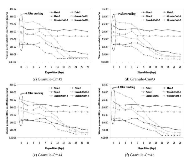
**Figure 9.** Water permeability coefficient on each crack width range in each mixture (1: <0.1 mm; 2: 0.1–0.2 mm; 3: >0.2 mm): (a) Granule-EA (CSA-based expansive agent); (b) Granule-Cm#1; (c) Granule-Cm#2; (d) Granule-Cm#3; (e) Granule-Cm#4; and (f) Granule-Cm#5.
