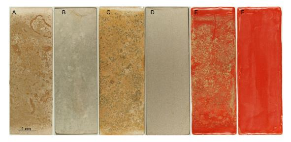
**Figure 1.** Photographs, showing the specimen surfaces after the three-month test. (**A**,**B**) 254SMO; (**C**,**D**) Ti alloy; (**E**,**F**) Inerta160-coated steel. Non-chlorinated: (**A**,**C**,**E**); chlorinated: (**B**,**D**,**F**).
