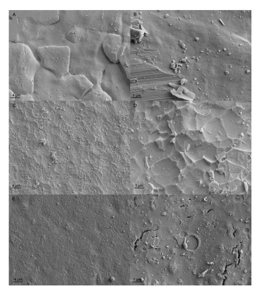
**Figure 4.** SEM images, showing the surface of coupons from the chlorinated system after three months of exposure. (**A**,**B**) SMO254; (**C**,**D**) Ti alloy; (**E**,**F**) Inerta160.
