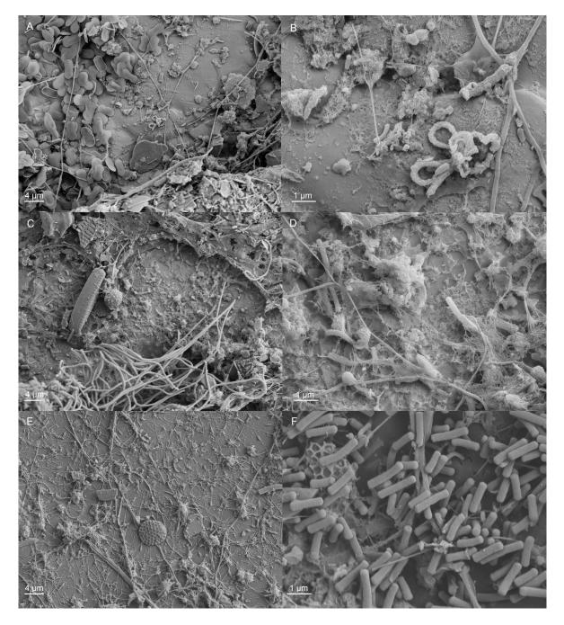
**Figure 3.** SEM images, showing the surfaces of coupons from the non-chlorinated system after three months of exposure. (**A**,**B**) 254SMO; (**C**,**D**) Ti alloy; (**E**,**F**) Inerta160.
