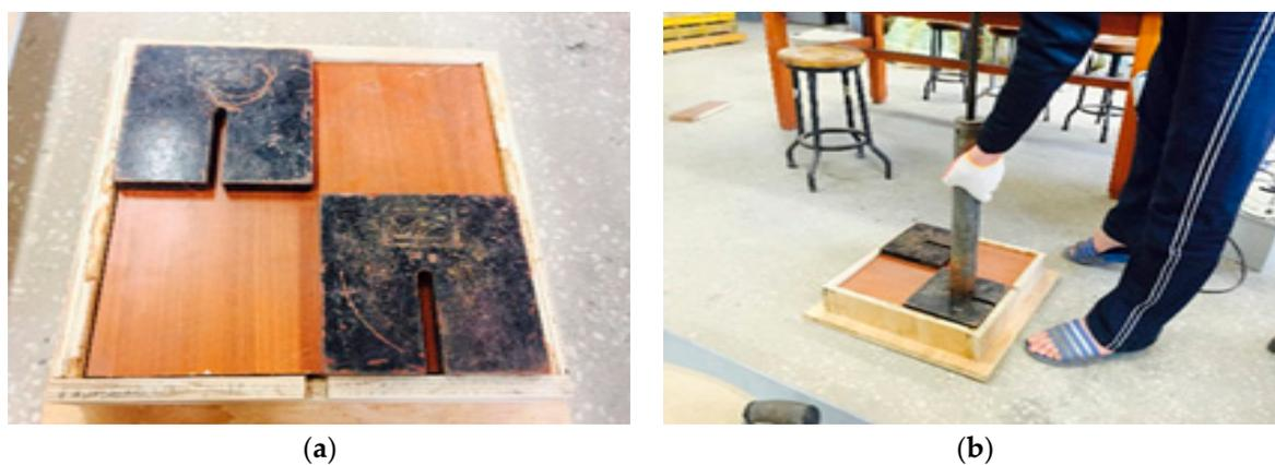
Figure 16. Compaction process. (a) Preparation of soil compaction with weight; (b) Compaction.
