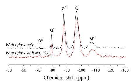
**Figure 5.** Liquid-state <sup>29</sup>Si NMR spectrum of waterglass and solid-state <sup>29</sup>Si MAS NMR spectrum of waterglass mixed with Na<sub>2</sub>CO<sub>3</sub>.
