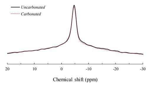
Figure 3. <sup>23</sup>Na MAS NMR spectra of uncarbonated and carbonated alkali-activated fly ash.
