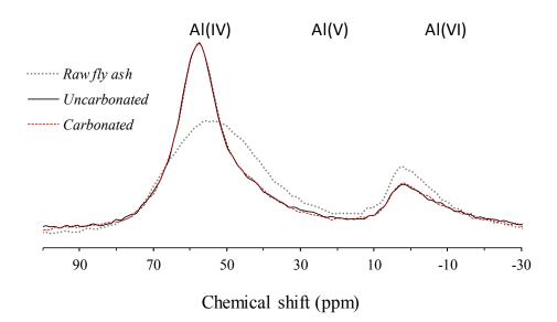
**Figure 2.** <sup>27</sup>Al MAS NMR spectra of raw fly ash and uncarbonated and carbonated alkali-activated fly ash.
