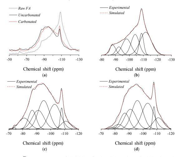
**Figure 1.** <sup>29</sup>Si MAS NMR spectra of (**a**) all; (**b**) raw fly ash; and (**c**) uncarbonated and (**d**) carbonated alkali-activated fly ash.
