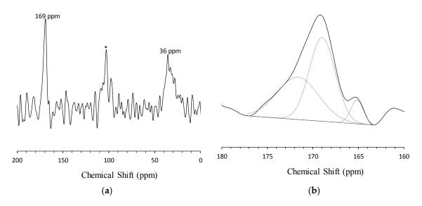
**Figure 4.** <sup>13</sup>C MAS NMR spectrum of carbonated alkali-activated fly ash. Spectral range of (**a**) 200 ppm to 0 ppm and; (**b**) 180 ppm to 160 ppm. The spinning sideband is marked with an asterisk.
