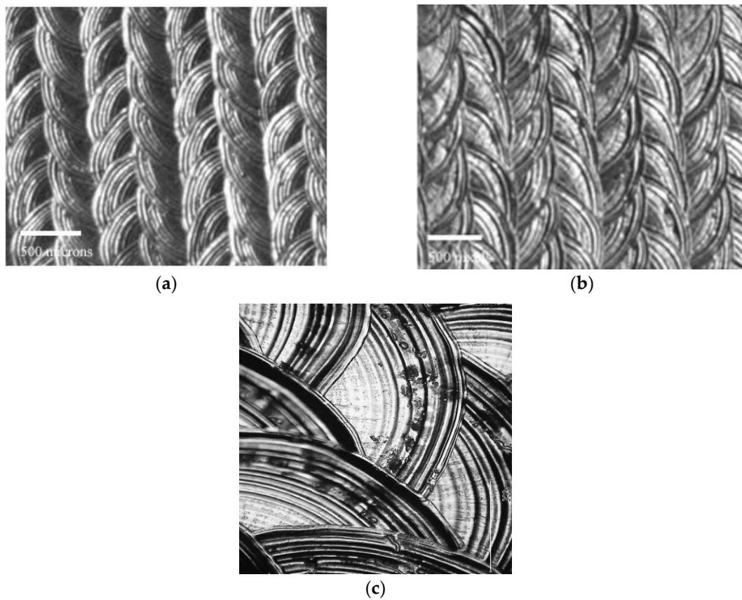
**Figure 6.** Surface features of the re-melted layers for different laser pulse power. (a) Surface topography of the sample re-melted with 2200 W laser pulse power; (b) Surface topography of the sample re-melted with 2600 W laser pulse power; and (c) magnified image of the surface topography of the sample re-melted with 2600 W laser pulse power.
