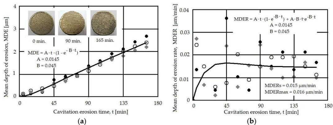
**Figure 8.** Cavitation erosion curves for the 2200 W laser pulse power. (a) Mean depth of erosion (MDE)( $t$ ); (b) Mean depth of erosion rate (MDER)( $t$ ).
