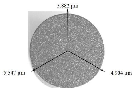
**Figure 1.** Macroscopic image of the Al<sub>2</sub>O<sub>3</sub>·30(Ni<sub>20</sub>Al) plasma deposited layer on the surface of CuAl10Ni5Fe2.5Mn1 sample (15.8 mm diameter) with the measured Rz data. Average Rz: 0.063  $\mu\text{m}$  for the polished base material; and 5.445  $\mu\text{m}$  for the plasma deposited layer.
