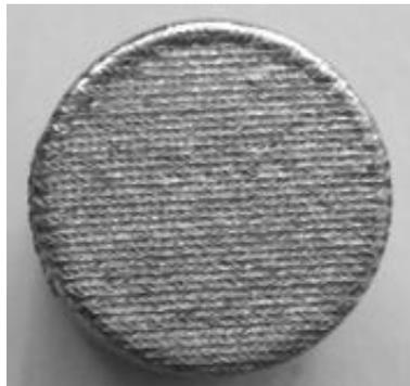
**Figure 4.** Macroscopic details of the surface of the laser re-melted sample prior to the cavitation erosion experiments (15.8 mm sample diameter).
