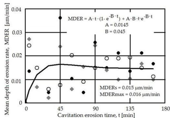
**Figure 11.** Comparative image of cavitation erosion resistance (reflected by the MDE *vs.* cavitation erosion time), indicating the improvement as a result of the alumina coating. The 2200 and 2600 W denote the parameters used for laser re-melting of the surface layer, following the  $\text{Al}_2\text{O}_3 \cdot 30(\text{Ni}_{20}\text{Al})$  plasma spraying. AMPCO 45 is the base metal shown for comparison purposes.
