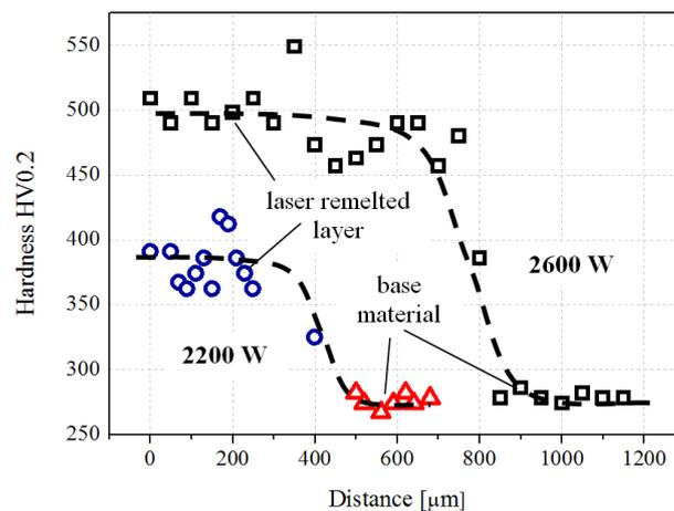
**Figure 7.** Hardness difference between the surface layer and the base materials (for 2200 W pulse power) and hardness profile across the interface (for 2600 W pulse power).
