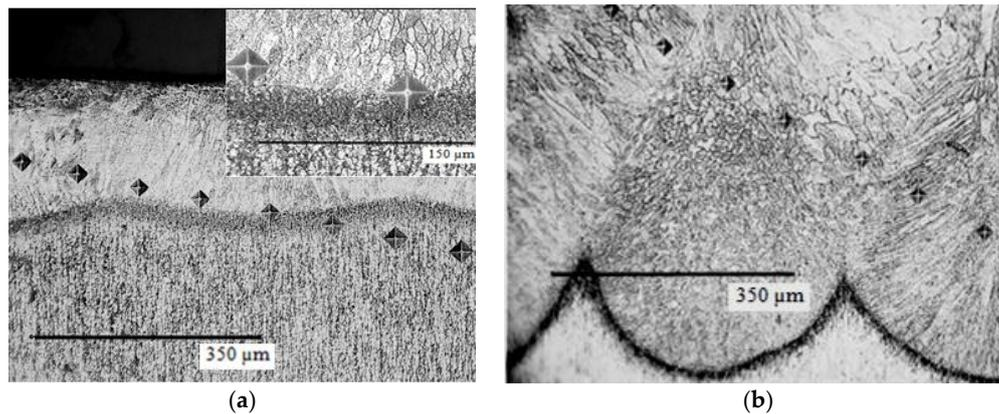
**Figure 5.** Cross-sectional microscopic details of the re-melted layer-substrate interface for different laser pulse powers. (a) Microstructure of the sample re-melted with 2200 W laser pulse power; and (b) microstructure of the sample re-melted with 2600 W laser pulse power.
