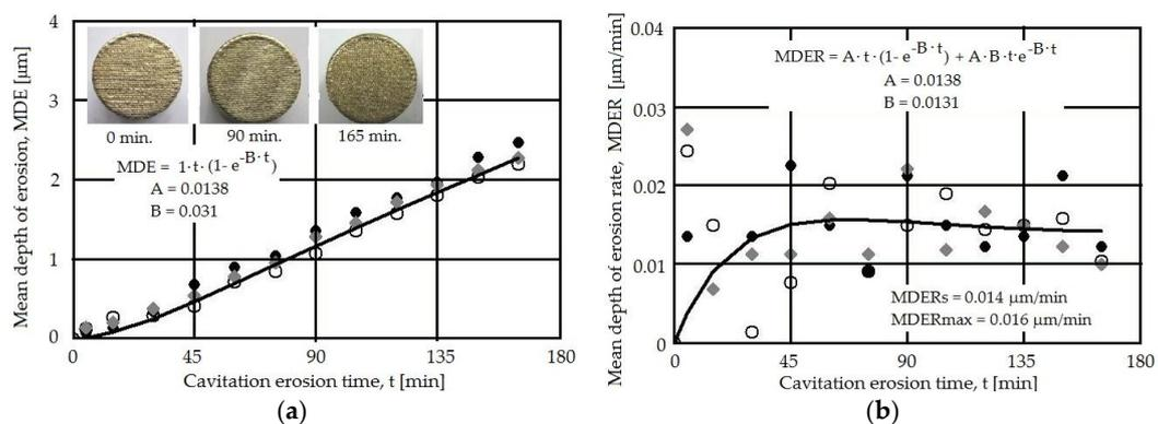
**Figure 9.** Cavitation erosion curves for the 2600 W laser pulse power. (a) MDE( $t$ ); and (b) MDER( $t$ ).
