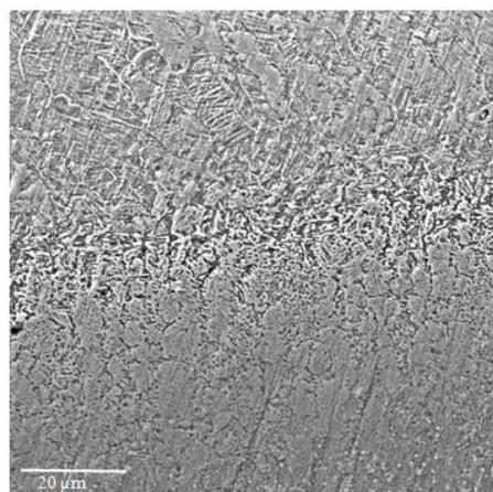
**Figure 2.** Details of the interface between the base materials and the plasma-deposited layer.
