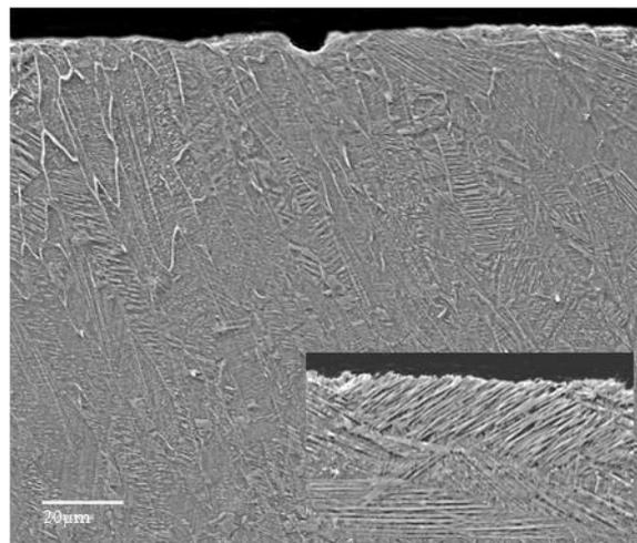
**Figure 10.** Cross-sectional details of the cavitation erosion effects. The inset shows the acicular substructure.
