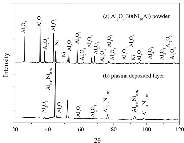
**Figure 3.** Comparative X-ray diffraction spectra of the  $\text{Al}_2\text{O}_3 \cdot 30(\text{Ni}_{20}\text{Al})$  powder and of the resulting plasma-deposited layer on the surface of the CuAl10Ni5Fe2.5Mn1 sample. (a) Diffraction spectrum for  $\text{Al}_2\text{O}_3 \cdot 30(\text{Ni}_{20}\text{Al})$  powder; (b) Diffraction spectrum for plasma deposited layer
