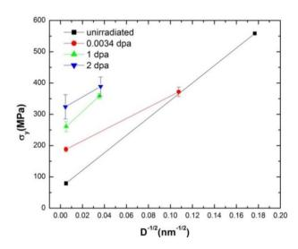
Figure 28. Variation of yield stress with grain size at all exposure level.
