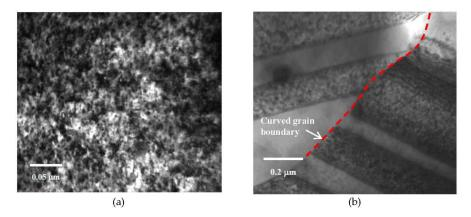
**Figure 14.** Bright field TEM images of MG-copper at 2 dpa showing formation of (**a**) high dislocation density; and (**b**) twin structures in a grain with curved boundary.
