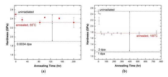
**Figure 27.** Variation of hardness of nc-copper with annealing time at (**a**) 55  $^{\circ}$ C; and (**b**) 100  $^{\circ}$ C, with dashed lines indicating the hardness of the material under the marked conditions.
