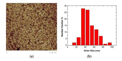
**Figure 8.** (a) AFM micrograph of as-received nc-copper; and (b) corresponding GSD showing variation in grain size between 10 and 100 nm with average grain size  $\sim$ 48 ± 16 nm.
