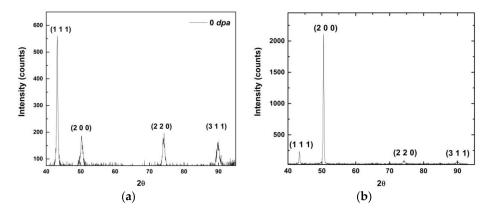
Figure 7. XRD patterns with major reflection peaks identified for (a) nc-copper; and (b) MG-copper.
