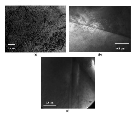
**Figure 13.** Bright field TEM micrographs of MG-copper at 1 dpa showing (**a**) dislocations in the grain interior; (**b**) dislocations at the grain boundary; and (**c**) twin structure.
