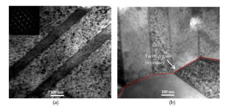
**Figure 20.** Bright field TEM of nc-copper at 1 dpa showing (**a**) formation of twin and dislocation structures; and (**b**) twin structures formed at a faceted grain boundary.
