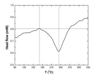
Figure 26. DSC scan of 3 mm disk of as-received nc-copper at heating rate of 10 K/min.
