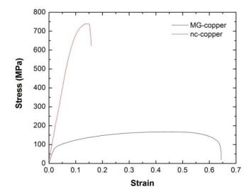
**Figure 10.** Engineering stress-strain curves of as-received MG and nc-copper from tensile testing at room temperature and strain rate of  $10^{-5} \cdot s^{-1}$ .
