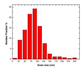
**Figure 19.** Grain size distribution (GSD) of irradiated nc-copper at 0.0034 dpa showing average grain size  $\sim$ 86  $\pm$  38 nm.
