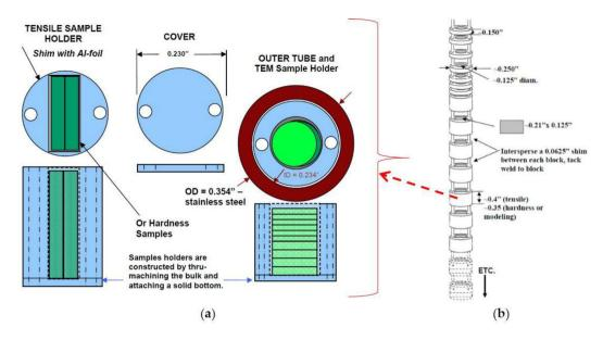
**Figure 3.** (**a**) Sample holder design for the ATR irradiation experiment; (**b**) schematic of the vertically stacked aluminum block sample holders in the test train assembly.
