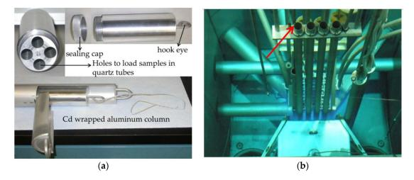
**Figure 1.** (a) Sample containment and Cd-wrapped aluminum column for neutron irradiation in PULSTAR; and (b) PULSTAR core with arrow indicating the WREP irradiation site.
