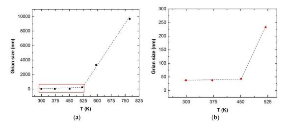
**Figure 24.** Variation of grain size of nc-copper with annealing temperature showing (**a**) sudden change in grain growth rate at ~520 K; and (**b**) onset of thermal instability at ~450 K.
