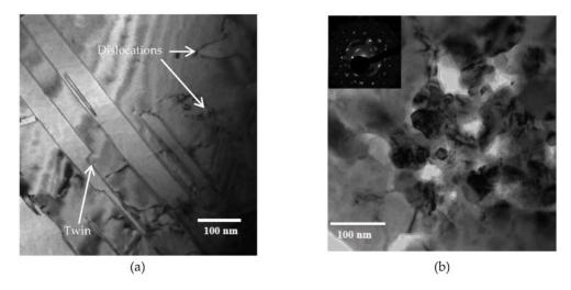
**Figure 18.** Bright field TEM of nc-copper at 0.0034 dpa showing (**a**) formation of both complete and incomplete twin and dislocation structures; and (**b**) population of grains with dimeter <100 nm.
