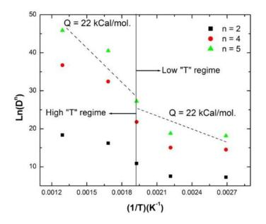
Figure 25. Arrhenius plot analyzing thermally-activated grain growth in as-received nc-copper.
