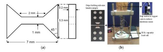
**Figure 5.** (a) Schematic of sub-size tensile sample; (b) photograph of the miniature tensile tester for mechanical loading of sub-size tensile samples.
