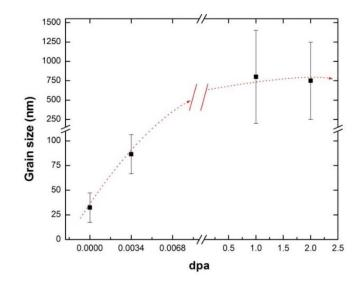
**Figure 23.** Variation of the average grain size of irradiated nc-copper with exposure level, showing grain growth at 0.0034 dpa and minimal change in average grain size between 1 and 2 dpa.
