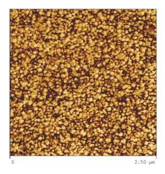
**Figure 17.** AFM image of nc-copper post 0.0034 irradiation with an average grain size of  $65 \pm 10$  nm.
