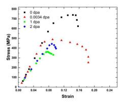
Figure 15. Representative engineering stress-strain curves of irradiated nc-copper.
