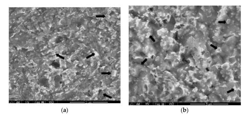
**Figure 22.** SEM images of irradiated nc-copper at (**a**) 1 dpa; and (**b**) 2dpa with arrows pointing at typical grains considered for grain size measurements.
