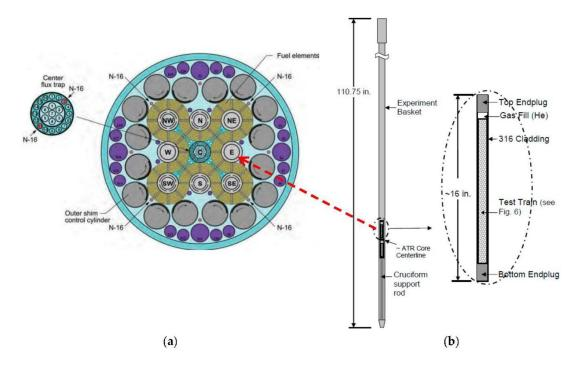
**Figure 2.** (a) Cross section view of ATR core with an arrow indicating irradiation test position E-7; (b) schematic of the irradiation test assembly for the ATR East Flux Trap Position.
