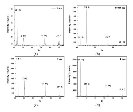
Figure 16. XRD patterns of nc-copper (a) as-received; (b) at 0.0034 dpa; (c) at 1 dpa; and (d) at 2 dpa.
