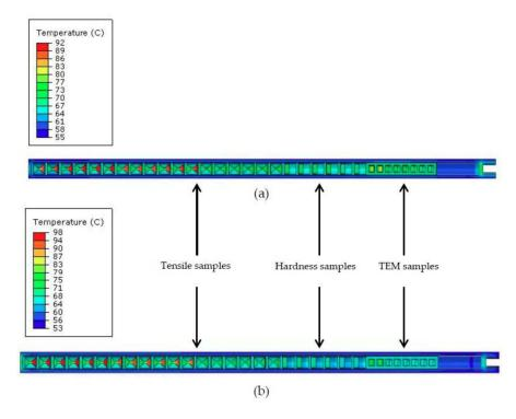
**Figure 4.** Irradiation temperature of copper samples as calculated by finite element model using Abaqus code in capsule irradiated up to (**a**) 1 dpa; and (**b**) 2 dpa.
