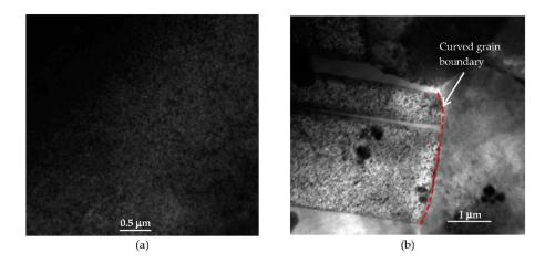
**Figure 21.** Bright field TEM of nc-copper at 2 dpa showing (**a**) formation of dislocation structures; and (**b**) twin structures formed at a curved grain boundary.
