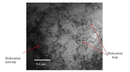
**Figure 12.** Bright field TEM micrograph of MG-copper at 0.0034 dpa showing dislocation loops and networks in the grain interior.
