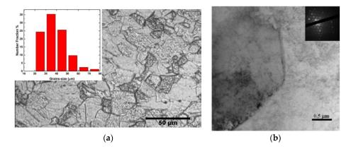
**Figure 6.** (a) Optical micrograph of as-received MG-copper with corresponding GSD inset showing average grain size  $\sim$ 38  $\pm$  12  $\mu$ m; and (b) Bright field TEM of as received MG-copper, with the corresponding diffraction pattern inset.
