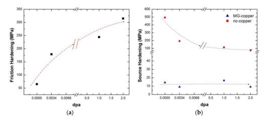
**Figure 29.** Variation of (**a**) friction hardening; and (**b**) source hardening of polycrystalline copper with exposure level.
