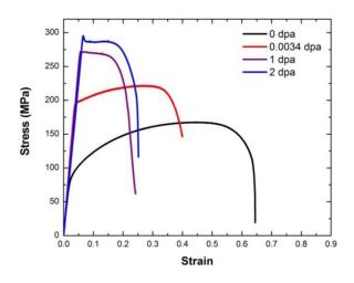
Figure 11. Engineering stress-strain curves of irradiated MG-copper.
