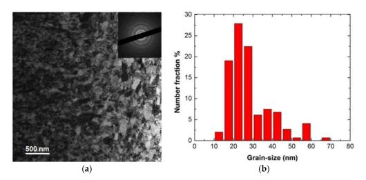
**Figure 9.** (a) Bright field TEM of as-received nc-copper; and (b) corresponding GSD with average grain size  $\sim 28 \pm 11$  nm.
