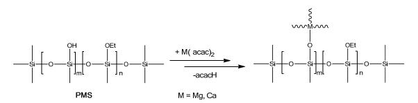
**Figure 1.** Sketch of the synthesis of the single-source precursor for SiCaMgOC upon chemical modification of PMS with acetyl acetonates of Ca and Mg.
