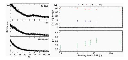
**Figure 2.** (a) XRD patterns of as-prepared SiOC powders (**bottom**) as well as after soaking in SBF [28] at 37 °C for 14 h (**middle**) and 15 days (**top**); (b) evolution of the content of Ca, Mg, and P in SBF (**above**) and pH (**below**) as a function of the soaking time during the SBF exposure of SiOC powders.
