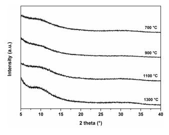
Figure 3. Diffraction patterns of SiCaMgOC glass pyrolyzed at 700, 900, 1100, and 1300 °C.
