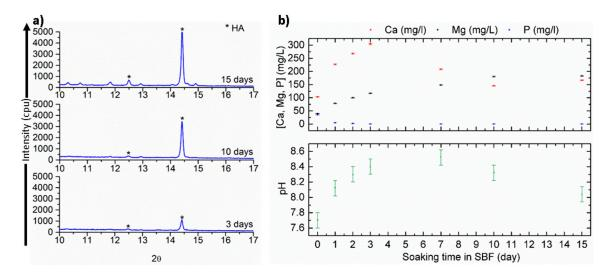
**Figure 4.** (a) XRD patterns of SiCaMgOC-1100 after soaking in SBF for 3, 10, and 15 days; (b) evolution of the Ca, Mg, and P contents in SBF (**above**) and pH (**below**) as a function of soaking time during the exposure of SiCaMgOC-1100 powder samples at 37 °C.
