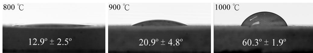
**Figure 3.** Water contact angles of Ti samples sintered at 800, 900, and 1000 °C in air.
