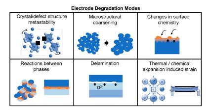
Figure 2. Illustration of degradation modes in oxygen electrode of SOFC/SOEC.
