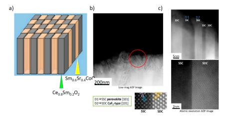
**Figure 3.** (a) Schematic of a double columnar oxygen electrode interlayer containing columns of  $Ce_{0.8}Sm_{0.2}O_2$  and  $Sm_{0.6}Sr_{0.4}CoO_3$  (b) TEM image of the prepared double columnar structure (c) High resolution TEM image. Taken with permission from [31] by Ju et al., with one modification: scale bar labels have been enlarged in this version for clarity.
