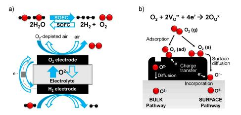
**Figure 1.** (a) Schematic of reversible solid oxide fuel/electrolysis cell; (b) two possible oxygen incorporation and reduction pathways in the oxygen electrode (SOFC mode).
