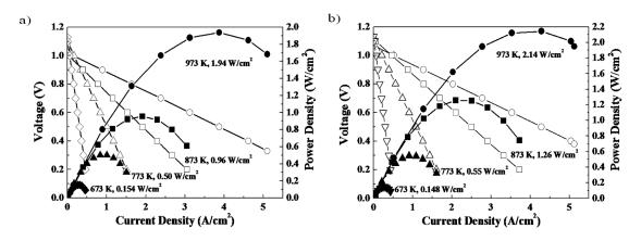
**Figure 4.** I-V and I-P curves of the cell using (**a**)  $Sm_{0.5}Sr_{0.5}CoO_3$  porous electrode fabricated from powder; (**b**) added  $Sm_{0.5}Sr_{0.5}CoO_3/Ce_{0.8}Sm_{0.2}O_2$  double columnar interlayer between the electrode and electrolyte. LSGM and Ni-Fe (9:1) were used for the electrolyte and fuel electrode, respectively. Taken with permission from [31] by Ju et al.
