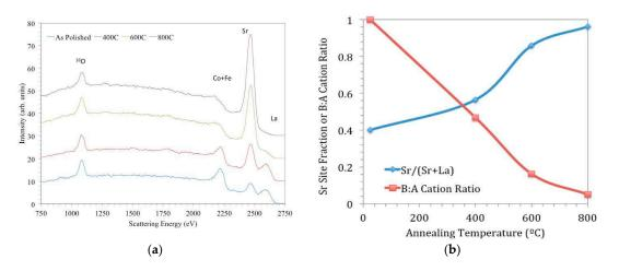
**Figure 10.** (a) LEIS spectra using 3 keV  ${}^{4}$ He ${}^{+}$  primary beam for LSCF ceramics annealed for 8 h at various temperatures. Adapted from [97] by Druce et al. with permission from Elsevier; (b) Fraction of Sr on A-site and B:A cation ratio quantified from spectra in (a).
