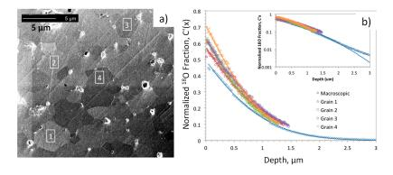
**Figure 8.** Depth profiling within individual grains in a polycrystalline LSCF sample exchanged at 450 °C in <sup>18</sup>O-enriched O<sub>2</sub> gas for 3721 s, using focused ion beam-secondary ion mass spectrometry (FIB-SIMS). (a) Microstructure, showing analyzed areas by ion-induced secondary electron image. Number labels in (a) identify grains from which the profiles plotted in (b) were obtained. Reprinted with permission of The Electrochemical Society, from [90] by Druce et al.
