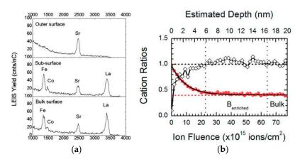
**Figure 11.** LEIS measurements with <sup>20</sup>Ne<sup>+</sup> primary beam at 6 keV at different depths of an LSCF ceramic annealed for 12 h at 1273 K. (a) Selected partial spectra corresponding to the very outer surface, the sub-surface and "bulk" regions; (b) Depth profile of Sr site fraction (solid circles) and B:A cation ratio (open diamonds). Reproduced from [98] by Druce et al. with permission of The Royal Society of Chemistry.
