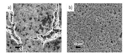
**Figure 12.** Scanning electron microscopy (SEM) images of LSCF cathodes exposed to different concentrations of sulfur impurity in the gas stream during electrochemical measurements of the degradation process, (**a**) 1513 ppm S; (**b**) 752 ppm S. Taken with permission from Elsevier, from [105] by Xie et al.
