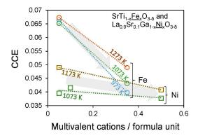
**Figure 6.** Coefficients of chemical expansion, CCEs, as a function of multivalent cation concentration per formula unit, i.e., *x* in  $\text{SrTi}_{1-x}\text{Fe}_x\text{O}_{3-\delta}$  and in  $\text{La}_{0.9}\text{Sr}_{0.1}\text{Ga}_{1-x}\text{Ni}_x\text{O}_{3-\delta}$  demonstrating correlation between charge delocalization and decreased CCEs. Data from [43,61] by Perry et al.
