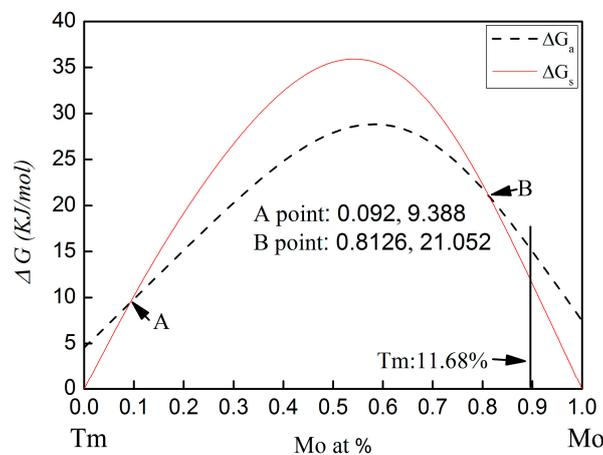
**Figure 5.** Gibbs free energy of the Mo-Tm system vs. molybdenum content.  $\Delta G_s$  and  $\Delta G_a$  are the Gibbs free energy of the crystalline solid solution and amorphization, respectively.
