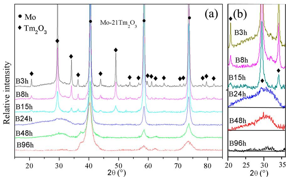
**Figure 1.** (a,b) X-ray patterns of Mo (21 wt %)  $\text{Tm}_2\text{O}_3$  powder mixtures milled for different times at a  $2\theta$  of  $15^\circ$ – $85^\circ$  and  $20^\circ$ – $36^\circ$ , respectively.
