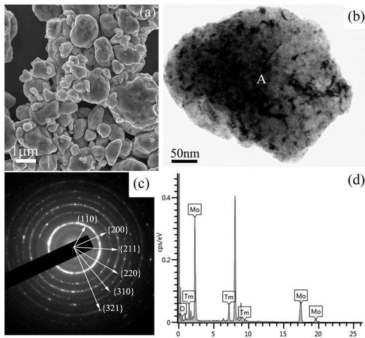
**Figure 3.** Microstructure analysis results of Mo (21 wt %)  $\text{Tm}_2\text{O}_3$  powder mixtures milled for 48 h; (a) SEM image showing the morphology of the ball-milled powders; (b) bright field TEM image; (c) selected area electron diffraction pattern from region 'A' in (a) showing the Mo phase; and (d) EDS analysis results from region 'A' in (a) showing the diffraction peaks of Tm, Mo, O, and Cu elements. Cu peaks comes from the copper grid.
