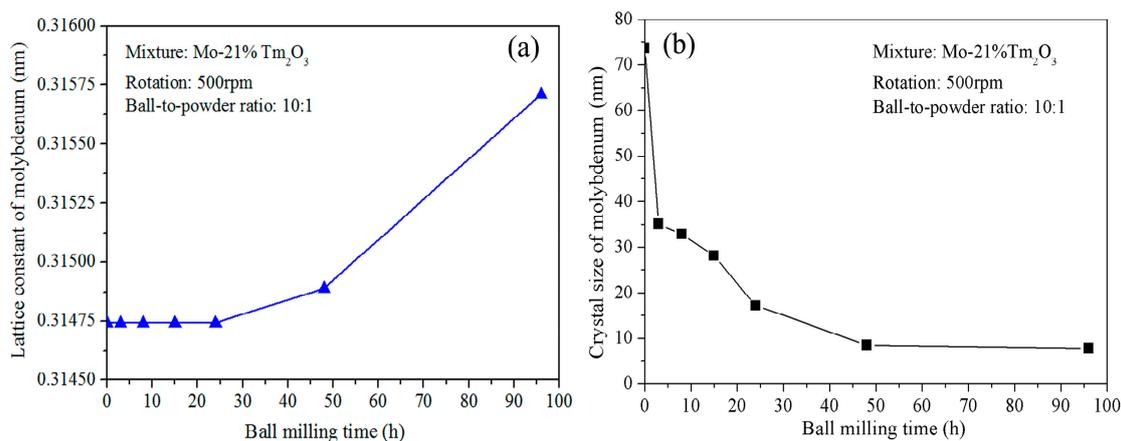
**Figure 2.** (a) Curve of the lattice parameter of Mo vs. ball-milling time; and (b) curve of the crystalline size of Mo vs. ball-milling time.
