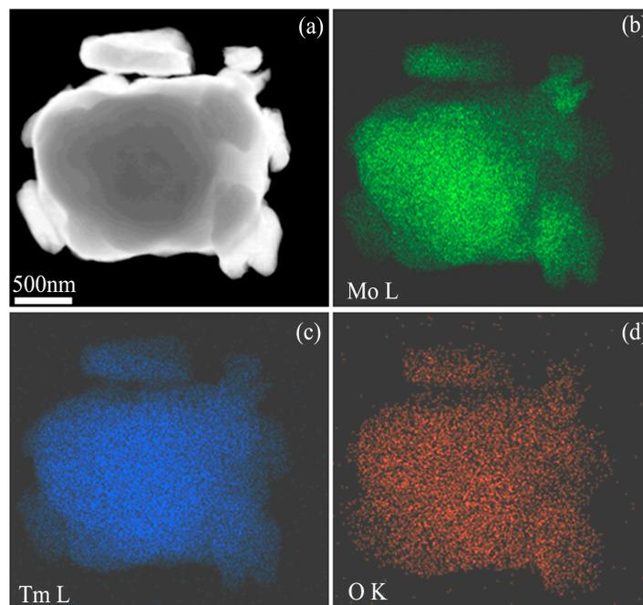
**Figure 4.** STEM analysis results of Mo (21 wt %)  $\text{Tm}_2\text{O}_3$  powder mixtures milled for 96 h; (a) high angle annular dark field STEM image; (b–d) Mo L, Tm L, and O K element mappings, respectively.
