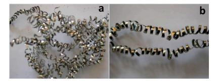
**Figure 12.** Optical images of tool wear and failure of  $Al_2O_3$ /TiAlN-coated insert ((**a**) under dry cutting; (**b**) under MQL; cutting time t = 12 min).
