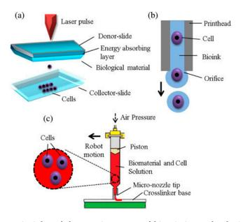
**Figure 2.** Working principles of three main groups of bioprinting technologies for tissue and organ engineering: (**a**) laser-based bioprinting; (**b**) inkjet-based bioprinting; and (**c**) extrusion-based bioprinting [22].
