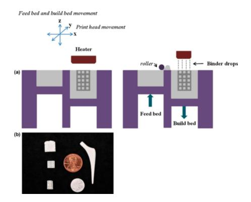
**Figure 3.** (a) 3D printing schematic using an inkjet printing system; and (b) 3D printed calcium phosphate (CaP) sintered structures fabricated at Washington State University using a 3D printer (ProMetal<sup>®</sup>, ExOne LLC, Irwin, PA, USA) [42].
