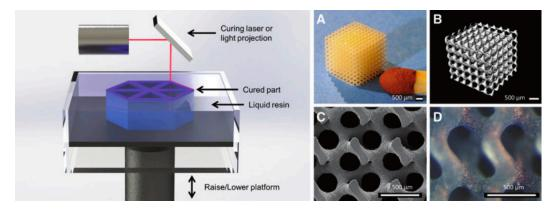
**Figure 4.** Schematic of stereolithographic (SLA) printing technique; and (**A**–**D**) exemplary tissue engineering scaffold composed of poly(D-L lactic acid) (PDLLA) that showcases the resolution and detail of SLA [47]: (**A**) photograph; (**B**) micro computed tomography (mCT); and (**C**,**D**) scanning electron microscope (SEM). Scale bar is 500 mm.
