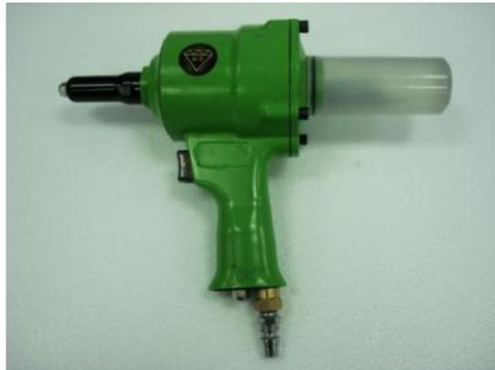
Figure 7. Pneumatic rivet gun.
