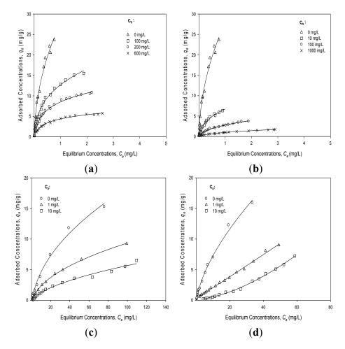
**Figure 3.** Single-solute and bi-solute isotherms of PHEN and DCP and NBZ on HBPMS and the fitting of the FM model: (a) PHEN isotherms with or without NBZ (at pH 7.0) as the competitor. (b) PHEN isotherms with or without DCP (at pH 7.0) as the competitor. (c) DCP isotherms with or without PHEN (at pH 7.0) as the competitor. (d) NBZ isotherms with or without PHEN (at pH 7.0) as the competitor.  $C_0$  (mg/L) is the added dose of the competitors.
