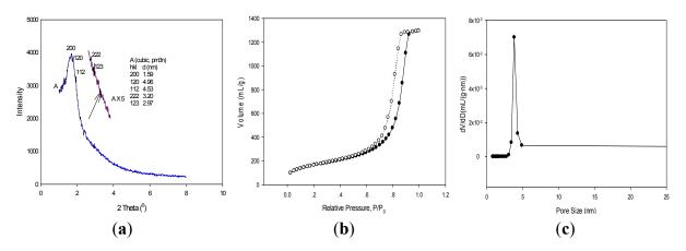
**Figure 1.** Small-angle X-ray diffraction (XRD) (**a**) nitrogen adsorption-desorption, (**b**) and pore size distribution (**c**) of the cubic Pm3n Hexylene-bridged periodic mesoporous polysilsesquioxanes (HBPMS). hkl: miller indices.
