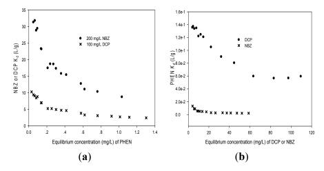
**Figure 4.** Competition between PHEN and neutral DCP and NBZ on HBPMS: (a)  $K_d$  of 200 mg/L NBZ or 100 mg/L DCP as a function of equilibrium PHEN concentration; (b)  $K_d$  of 10 mg/L PHEN as a function of equilibrium DCP or NBZ concentration.
