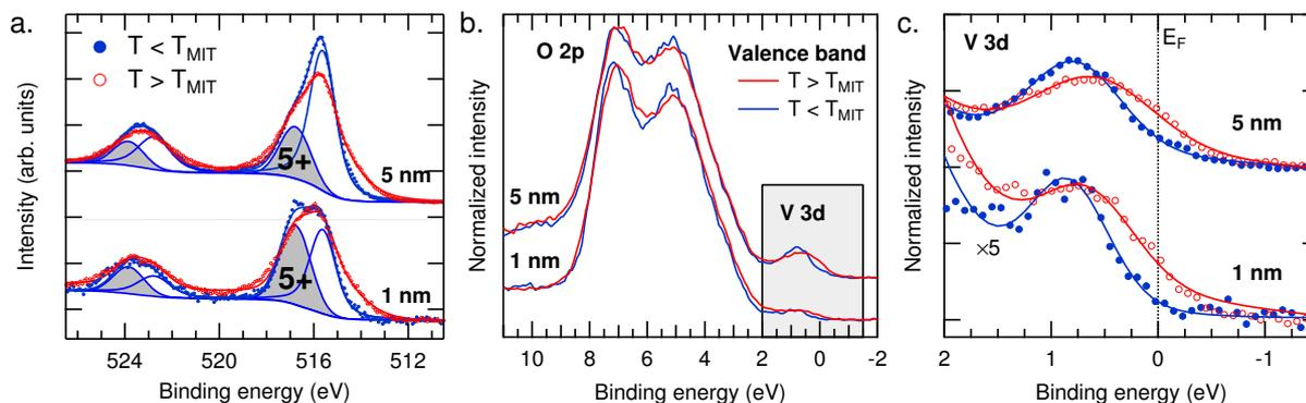
**Figure 6.** (a) V 2p HAXPES measured above (red) and below (blue)  $T_{MIT}$  for two  $\text{VO}_2/\text{TiO}_2$  (100) films with thickness of 5 nm and 1 nm, respectively. Peak fitting results are shown for the low temperature measurement; (b) Valence band HAXPES; and (c) an expanded view of the topmost V 3d states of the same two samples.
