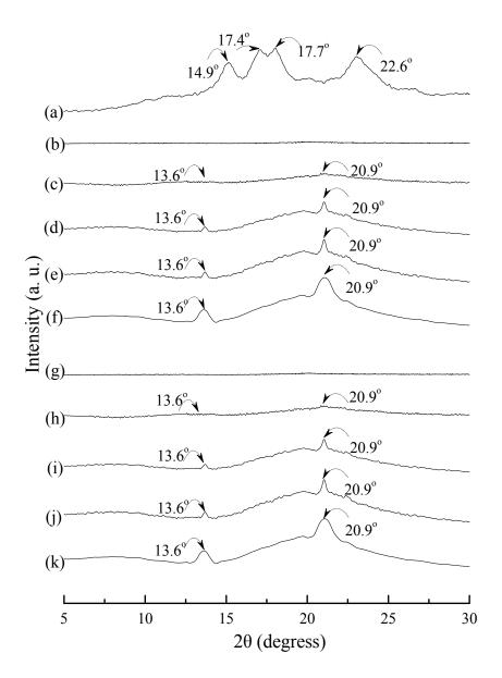
**Figure 8.** Wide-angle X-ray diffraction patterns of (a) tapioca, TPS specimens conditioned at 20 °C/50% RH for (b) 0; (c) 7; (d) 14; (e) 28 and (f) 56 days, respectively; and TPS<sub>100</sub>BC<sub>0.02</sub> specimens conditioned at 20 °C/50% RH for (g) 0; (h) 7; (i) 14; (j) 28 and (k) 56 days, respectively.
