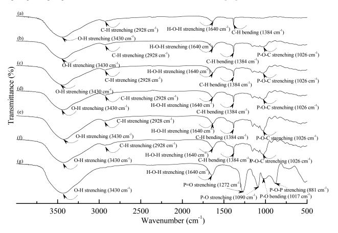
**Figure 1.** FTIR spectra of (**a**) TPS100BC0.02; (**b**) TPS100BC0.02SHMP4; (**c**) TPS100BC0.02SHMP8; (**d**) TPS100BC0.02SHMP10; (**e**) TPS100BC0.02SHMP16; (**f**) TPS100BC0.02SHMP32 and (**g**) SHMP specimens.
