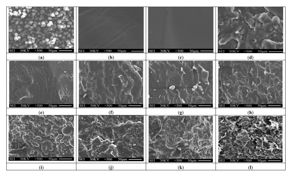
Figure 3. SEM micrographs of fracture surfaces of initial (a) Tapioca starch; (b) TPS; (c) TPS100BC0.02; (d) (TPS100BC0.02)75PLA25; (e) TPS100BC0.02SHMP4; (f) TPS100BC0.02SHMP8; (g) TPS100BC0.02SHMP10; (h) TPS100BC0.02SHMP16; (i) (TPS100BC0.02SHMP4)75PLA25; (j) (TPS100BC0.02SHMP8)75PLA25; (k) (TPS100BC0.02SHMP10)75PLA25 and (l) (TPS100BC0.02SHMP16)75PLA25 specimens.
