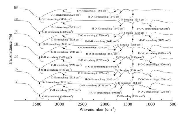
Figure 2. FTIR spectra of (a) PLA; (b) TPS100BC0.02SHMP4; (c) (TPS100BC0.02SHMP4)75PLA25;
