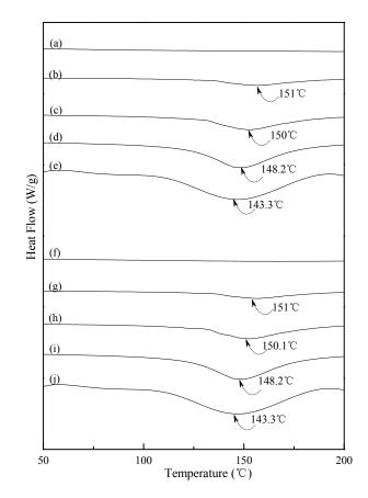
**Figure 5.** DSC thermograms of TPS specimens conditioned at 20 °C/50% RH for (**a**) 0; (**b**) 7; (**c**)14; (**d**) 28 and (**e**) 56 days, respectively; and TPS<sub>100</sub>BC<sub>0.02</sub> specimens conditioned at 20 °C/50% RH for (**f**) 0; (**g**) 7; (**h**) 14; (**i**) 28 and (**j**) 56 days, respectively.
