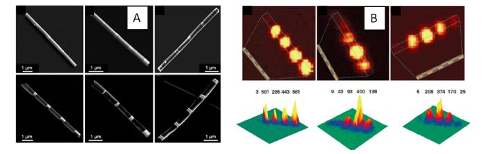
**Figure 6.** (A) SEM images of on-wire lithography (OWL)-generated nanodisk arrays with various geometries; (B) Confocal Raman microscopy images of gapped nanowire structures functionalized with methylene blue (MB) [104]. (Reproduced with permission from Qin *et al.*, published by National Academy of Sciences, USA, 2006.)
