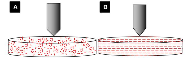
Figure 7. Schematic feature of fibers oriented (A) randomly (produced by right angle extruder);(B) organized perpendicular to direction of load (produced by 160° extruder).
