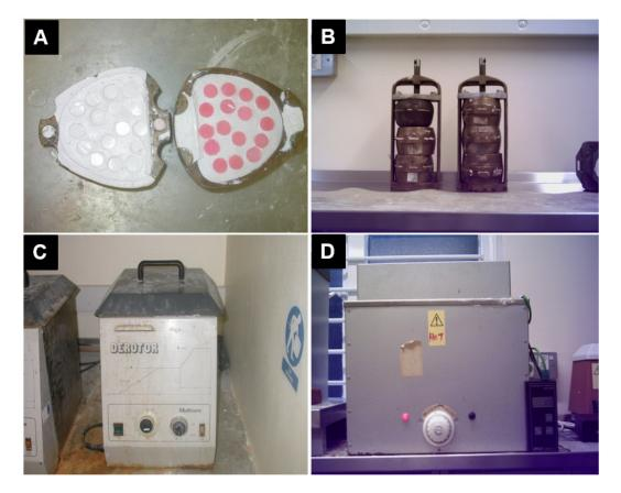
Figure 9. (A) Conventional method of flasking discs; (B) Conventionally packed and clamped flasks; (C) water bath (D) dry heat oven.
