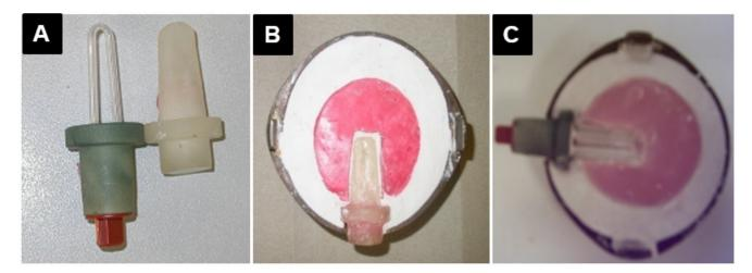
Figure 12. (A) Duplicated thermocouple head; (B) Investing the duplicated dummy; (C) Thermocouple head located inside the resin.
