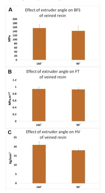
Figure 5. Effect of extruder angle on (A) BFS; (B) fracture toughness (FT); and (C) HV of veined PMMA. VIm W (veined type of resin packed using modified extruder,  $160^{\circ}$ , cured in the water bath), VIW (veined type of resin packed using standard extruder,  $90^{\circ}$ , cured in the water bath).
