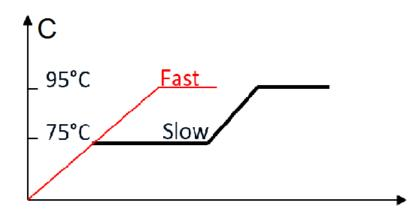
**Figure 6.** Pattern of temperature in (**A**) water bath loaded with 5 and 10 flasks and cure under slow (4 h 75 °C + 2 h 95 °C) and fast (2 h 95 °C) processing methods was measured; (**B**) Pattern of temperature inside the curing resin while water bath loaded with 5 flasks was measured; (**C**) Pattern of temperature in dry heat oven loaded with 0, 2, 5 and 10 flasks.
