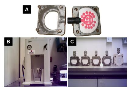
Figure 10. (A) Tree-shaped wax pattern invested in the flask with a plastic dummy;
