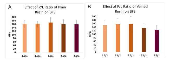
**Figure 3.** Effect of power/liquid ratio on BFS of (**A**) plain PMMA; and (**B**) veined PMMA for both plain and veined PMMA.
