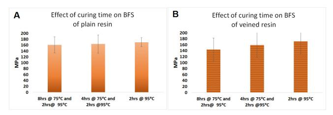
Figure 4. Effect of curing time in water bath on BFS of (A) plain and (B) veined PMMA.
