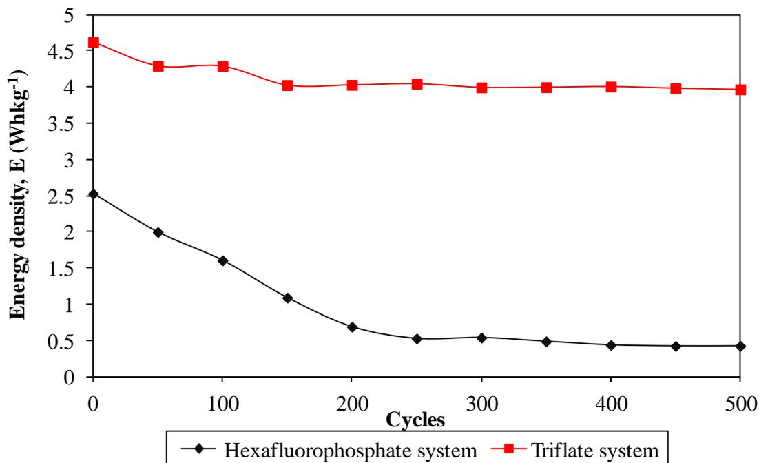
**Figure 11.** Power density of different ionic liquid-based biopolymer electrolyte systems over 500 cycles.
