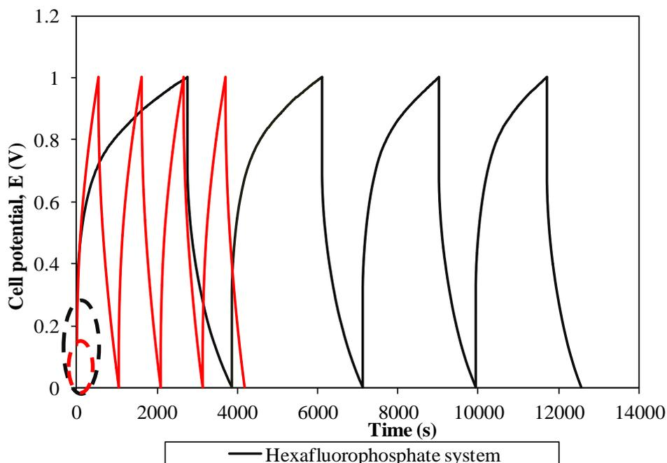
Furthermore, the electrochemical performance in terms of stability is investigated by charging and discharging the cells for 500 cycles. Figures 8–11 describe the specific capacitance, Coulombic efficiency, energy density and power density of both types of supercapacitors over 500 cycles, respectively. The specific capacitance and energy density of both cells decrease abruptly with increasing cycle number.
