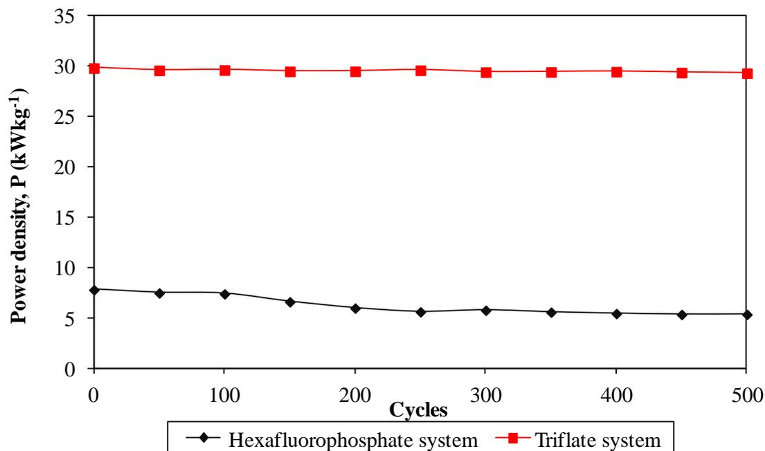
On the other hand, the power density of both cells reduces gradually as the charging and discharging cycle increase. Such reduction might be ascribed to the depletion of the polymer electrolytes and immobilization of the charge carriers after prolonged charge and discharge processes. However, the Coulombic efficiency of both cells increases with the cycle number. The triflate system shows an efficiency above 90% within 500 cycles, whereas the hexafluorophosphate system reveals
