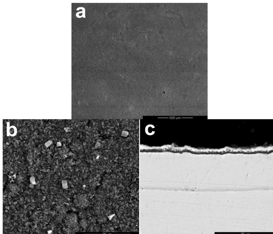
**Figure 4.** The (a) surface and (b) cross-sectional morphology of Y-enriched particle formed on the K38-0.5Y coating surface after 60 h at 900 °C.
