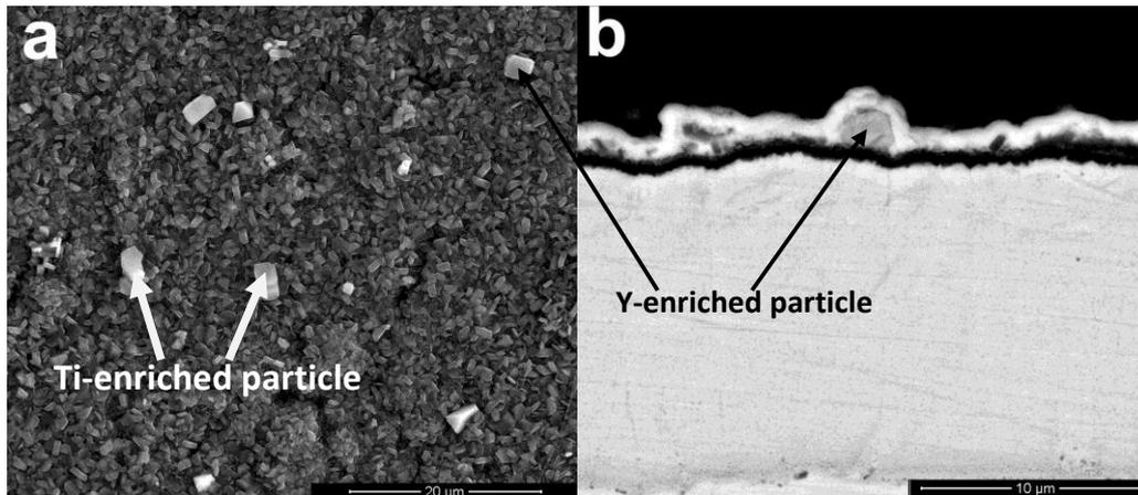
**Figure 5.** XRD Elemental mapping of the Y-enriched particle formed on the K38-0.5Y coating surface at 900 °C.
