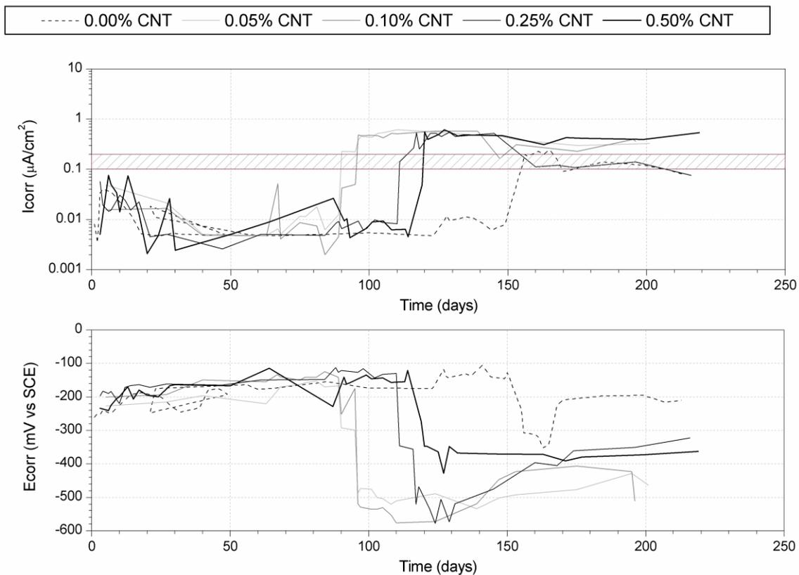
As a consequence of these two factors, it can be expected that the higher CNT dosage would lead to higher conductivity and therefore higher galvanic couple effect from the carbon material to the steel reinforcement. Finally, the complementary action of these two factors implies higher corrosion levels, which is consistent with the obtained results.
