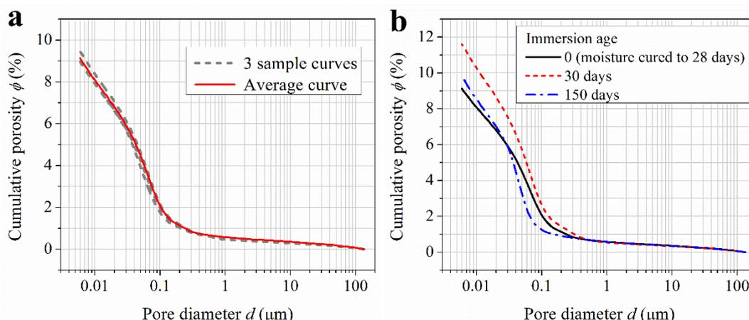
Diamond, who introduced MIP into concrete technology in 1970s, has pointed out that the MIP pore size distribution curve is far from realistic, and MIP results are valuable only to provide intrudable porosities and threshold pore diameters which can serve as porosity index and connectivity
