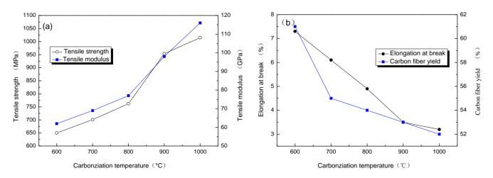
Higher weight losses, or lower yield result in higher production costs [15]. Figure 2b shows the yields of carbon fibers are 61%~52% from 600 to 1100 °C. It is clear that the yield of CBCFs is higher than that of carbon fibers produced from cellulose.
