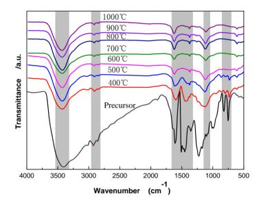
Figure 3. FTIR spectra of CBCFs at various temperatures.
