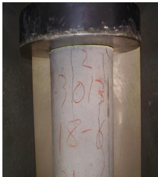
Due to the results discussed above, and considering that the structural panel to be manufactured must have a characteristic strength at 28 days of  $40 \text{ N/mm}^2$ , the viability of samples with 20% and 25% percentages of PCM are discarded because of lower strength.
