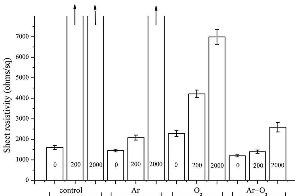
The sheet resistance data of PPy coated PVDF samples in Figure 6 and photographs of abraded samples in Figure 5 agree with each other and all confirm the order of plasma gas effectiveness as (Ar + O<sub>2</sub>) > O<sub>2</sub> > Ar. Contact angle measurements show an improvement in the PVDF surface wettability after the plasma treatment. The decrease of the F/C ratio and water contact angle prove that both chemical and physical effects play an important role in the adhesion.
