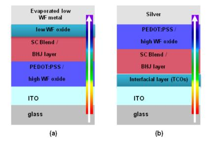
To overcome the instability issue in the normal structure device, one feasible approach is to construct an inverted configuration [2,30], where ITO serves as the cathode, as shown in Figure 2b.
