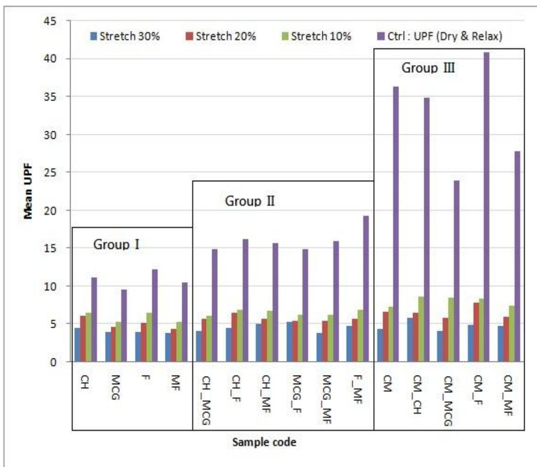
The pores are larger as the fabric is stretched more, as shown in Figure 5 (using “CH\_F” as an example). The magnitude of decrease in UPF is most profound in Group III, compared with Group II and Group I, as shown in Figure 4. As the presence of holes dominates the cause of decreasing UPF, effects of fibre type and the spinning method become insignificant and negligible in this Group.
