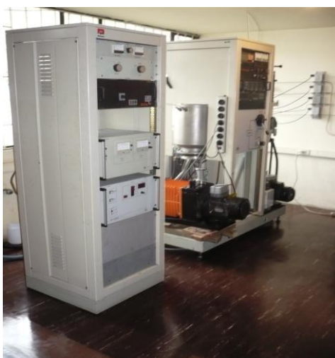
Figure 1. Alcatel HS 2000 RF sputtering system.
