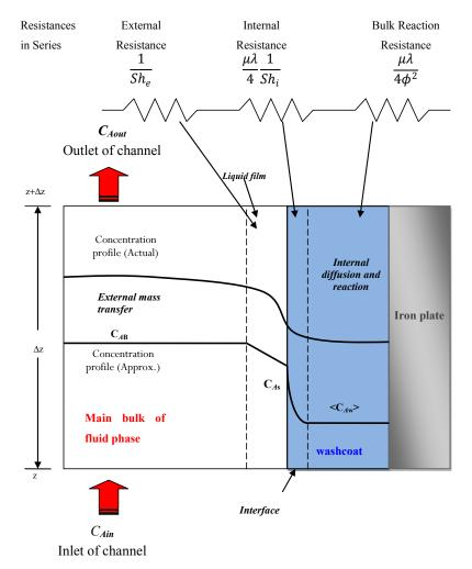
**Figure 1.** Schematic diagram of the control volume that illustrates the fluid-solid mass transfer during a chemical reaction in the washcoat with resistances using a series approach.
