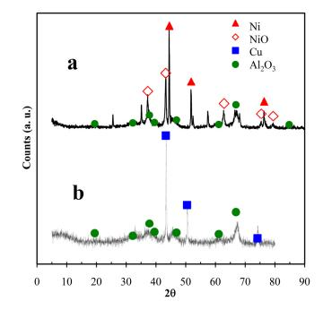
Figure 2. XRD patterns of prepared powders of (a) Ni; and (b) Cu particles on alumina.
