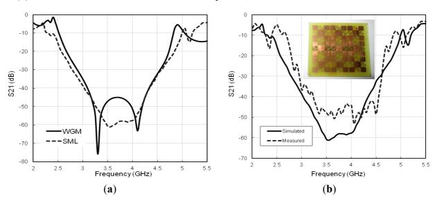
**Figure 4.** (a) Transmission responses of the MBHIES from two different methods; (b) Simulated and measured transmission responses,  $S_{21}$ .
