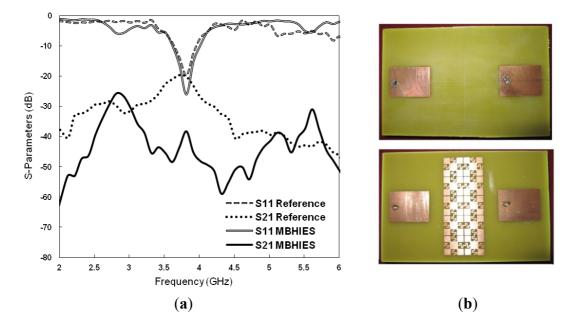
Figure 11. (a) Measured S-parameters of the microstrip antenna array; (b) fabricated prototypes.
