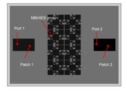
Prior to applying MBHIES to the antenna array, the mutual coupling effects are examined by varying the patch separation (D). Figure 7a plots the mutual coupling for various patch separations and Figure 7b plots the minimum coupling (in both E- and H-plane directions) for different distances at the resonant frequency of 3.8 GHz. It is clear from the figures that the coupling coefficient level degrades
