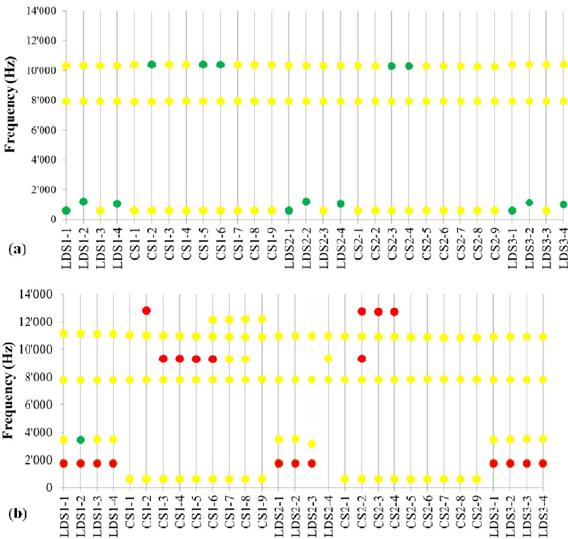
Figure 2. Frequencies and intensities of noise recorded during linear decreasing speed (LDS) and constant speed (CS) tests for: (a) Formulation 4 with 8% T800 graphite; (b) Formulation 5 with 8% T200-2000 graphite; (c) Formulation 6 with 4% T150-600 and 4% C-THERM TM 011 graphite. Green dots < 60\text{ dB} , 60 dB < yellow dots < 80\text{ dB} , red dots > 80\text{ dB} . The sequence of the test ( x -axis) is described in Table 2.
