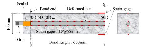
**Figure 3.** A specimen for the uniaxial tension test.
