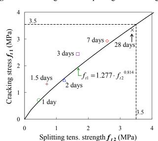
**Figure 10.** Cracking stress *vs.* splitting tensile strength.
