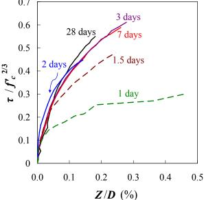
Figure 13 shows that the data obtained from the experiments can be expressed by using the empirical equation. The coefficient a represents the ultimate bond stress; it develops with age and becomes constant after the age of 2 days. Interestingly, the coefficient b of all the regression lines in the graph is approximately 0.12. The empirical equations may be useful for predicting the crack width of early age concrete, but they are limited to the mix proportions and materials used in the study.
