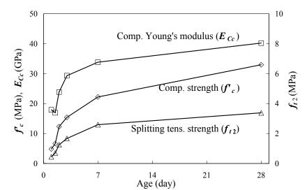
**Figure 2.** Compressive strength, splitting tensile strength and compressive Young's modulus.
