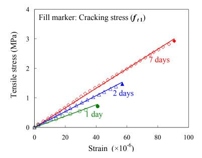
**Figure 8.** Tensile stress-strain responses (at the ages of 1, 2, 7 days).
