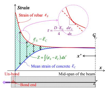
Mimura *et al.* used a similar equation for estimating the concrete strain, but that study employed compressive Young's moduli obtained from cylindrical specimens [25]. Tensile Young's moduli are more appropriate for estimating the tensile strain of concrete. Therefore this study uses the tensile modulus obtained in the previous chapter instead of the compressive modulus.
