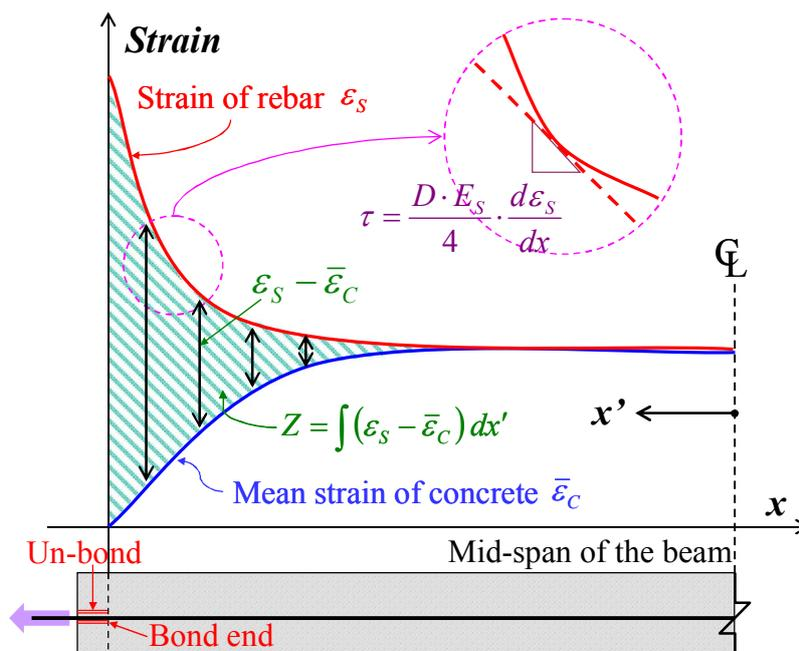
Mimura *et al.* used a similar equation for estimating the concrete strain, but that study employed compressive Young’s moduli obtained from cylindrical specimens [25]. Tensile Young’s moduli are more appropriate for estimating the tensile strain of concrete. Therefore this study uses the tensile modulus obtained in the previous chapter instead of the compressive modulus.
