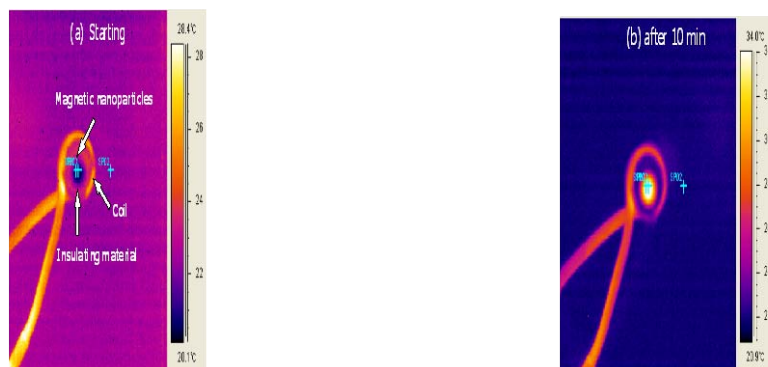
Figure 7. FLIR Thermacam ® images taken (a) at starting and (b) after 10 minutes for the heating of magnetic nanoparticles under a 653 Oe (266KHz) field.
