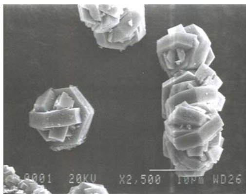
Figure 6. Electron micrograph of intergrown hexagonal troilite platelets.
