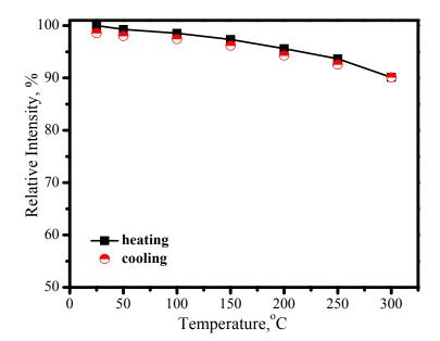
**Figure 19.** Luminescence intensity of  $(Lu_{0.9}Ce_{0.01})_3Al_5O_{13}$  as a function of temperature.
