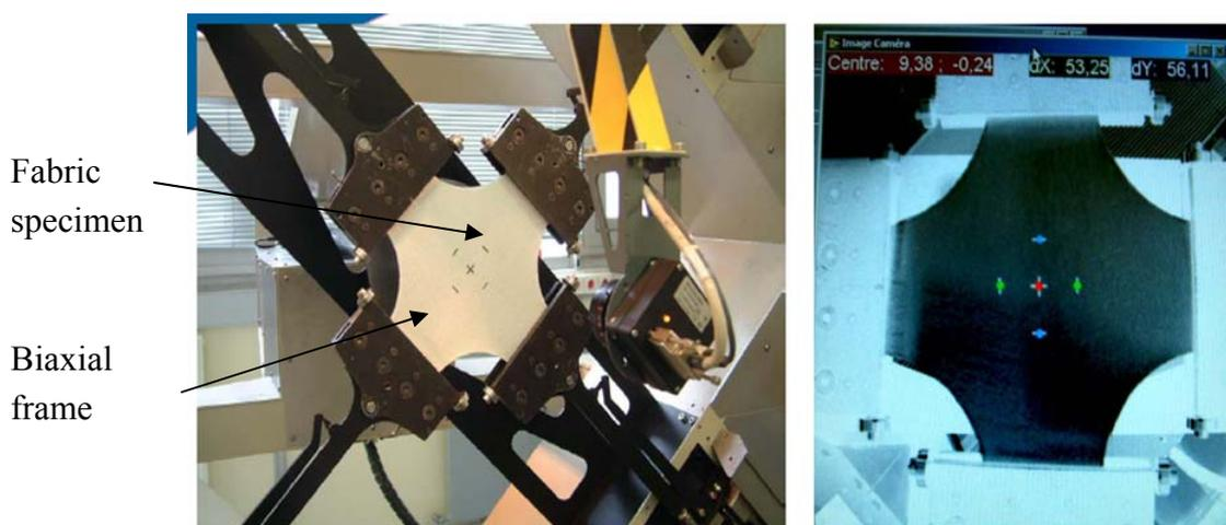
For a given fabric, the response is strongly influenced by the strain ratio in warp and weft directions due to large fibre undulations. Especially, the non-linearity in warp and weft direction is increasing. The tendency of the fibre to straighten is more impeded when the strain in the perpendicular direction is large (see Table 2). The biaxial specimen, as shown in Figure 9, was modelled in 2D with 400 four
