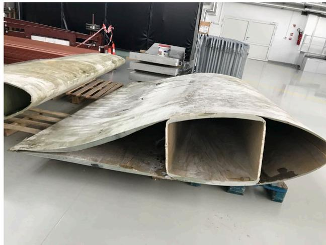
**Figure 4.** Sections cut from wind turbine blade.
