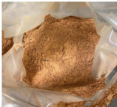
**Figure 3.** Ceramic fines after ball milling to fraction <0.063 mm.
