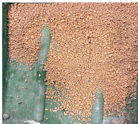
**Figure 2.** Aggregate received from crushing ceramic blocks, fraction 0–4 mm.
