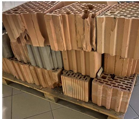
**Figure 1.** Ceramic blocks LPW 25 250/380/238 used in crushing process.
