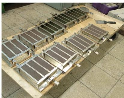
**Figure 5.** Preparation of geopolymer mortar samples.
