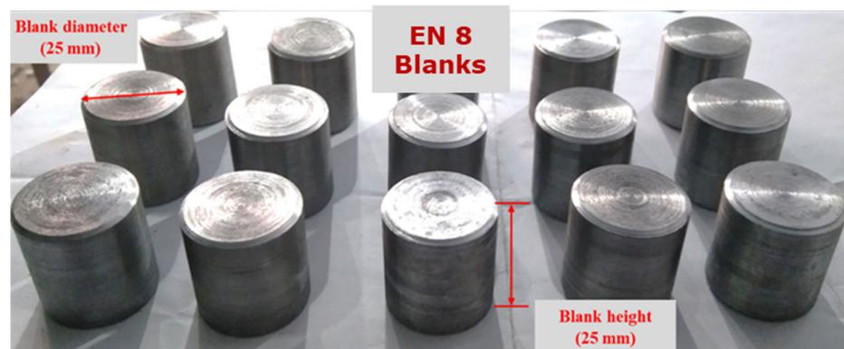
**Figure 2.** The EN8 steel cylindrical blanks used to fabricate rotors.
