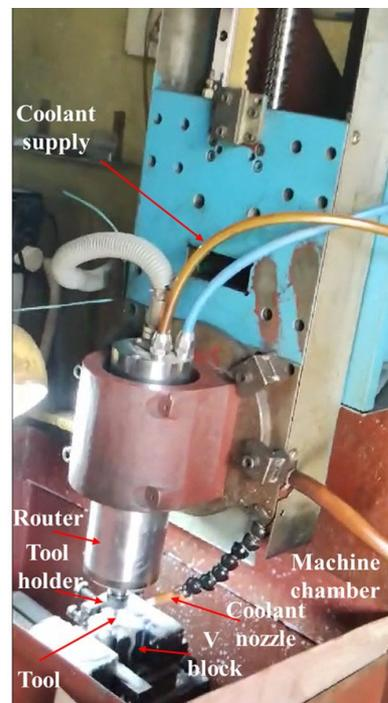
**Figure 1.** CNC engraving milling machine tool used in the present work.
