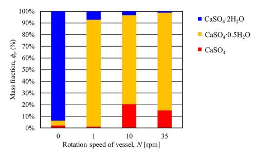
**Figure 15.** Relationship between the transferring mass fraction of gypsum and the rotation speed of the rotary vessel at a heating temperature of 180 °C.
