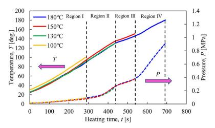
**Figure 2.** Time histories of temperature and pressure inside the rotary vessel.
