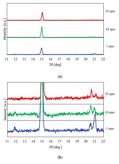
**Figure 14.** XRPD measurement results at a heating end temperature of  $180\,^{\circ}\text{C}$  when the rotation speed was changed; **(a)** Normal figure; **(b)** Enlarged figure.
