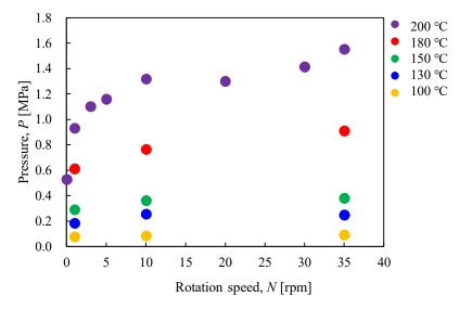
**Figure 18.** Relationship between the pressure in the rotary vessel and the rotation speed when the heating end temperature was changed.
