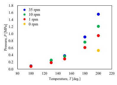
**Figure 17.** Relationship between the pressure in the rotary vessel and the heating end temperature when the rotation speed was changed.
