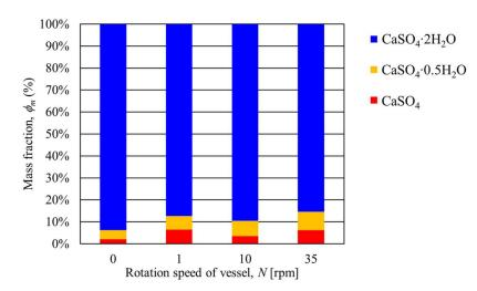
**Figure 6.** Relationship between the transferring mass fraction of gypsum and the rotation speed of the rotary vessel at a heating end temperature of  $100\,^{\circ}$ C.
