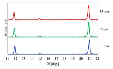
**Figure 5.** XRPD measurement results at a heating end temperature of 100  $^{\circ}$ C when the rotation speed was changed.
