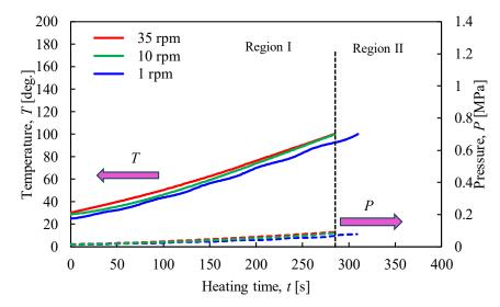
**Figure 4.** Time histories of temperature and pressure inside the rotary vessel at a heating end temperature of 100 °C when the rotation speed was changed.
