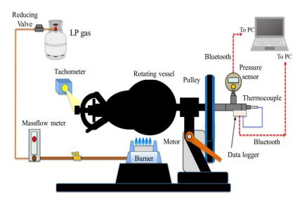
Figure 1. Material heating equipment using a constant-volume rotary vessel.
