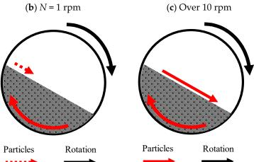
Figure 16. Typical flow pattern of gypsum particles in a rotating vessel.
