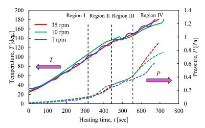
**Figure 13.** Time histories of temperature and pressure inside the rotary vessel at a heating end temperature of  $180 \,^{\circ}$ C when the rotation speed was changed.
