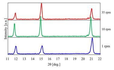
**Figure 11.** XRPD measurement results at a heating end temperature of 150  $^{\circ}$ C when the rotation speed was changed.
