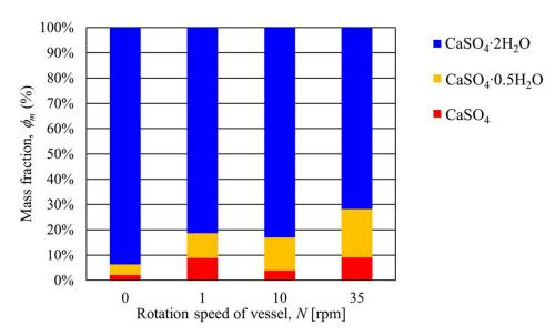
**Figure 9.** Relationship between the transferring mass fraction of gypsum and the rotation speed of the rotary vessel at a heating end temperature of 130 °C.
