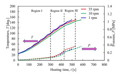
**Figure 10.** Time histories of temperature and pressure inside the rotary vessel at a heating end temperature of 150 °C when the rotation speed was changed.
