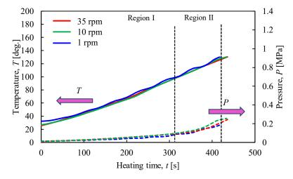
**Figure 7.** Time histories of temperature and pressure inside the rotary vessel at a heating end temperature of 130 °C when the rotation speed was changed.
