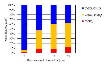
**Figure 12.** Relationship between the transferring mass fraction of gypsum and the rotation speed of the rotary vessel at a heating end temperature of  $150 \,^{\circ}$ C.
