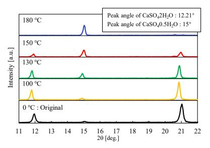
Figure 3. XRPD measurement results.
