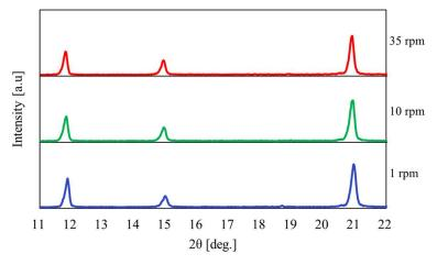
**Figure 8.** XRPD measurement results at a heating end temperature of 130  $^{\circ}$ C when the rotation speed was changed.
