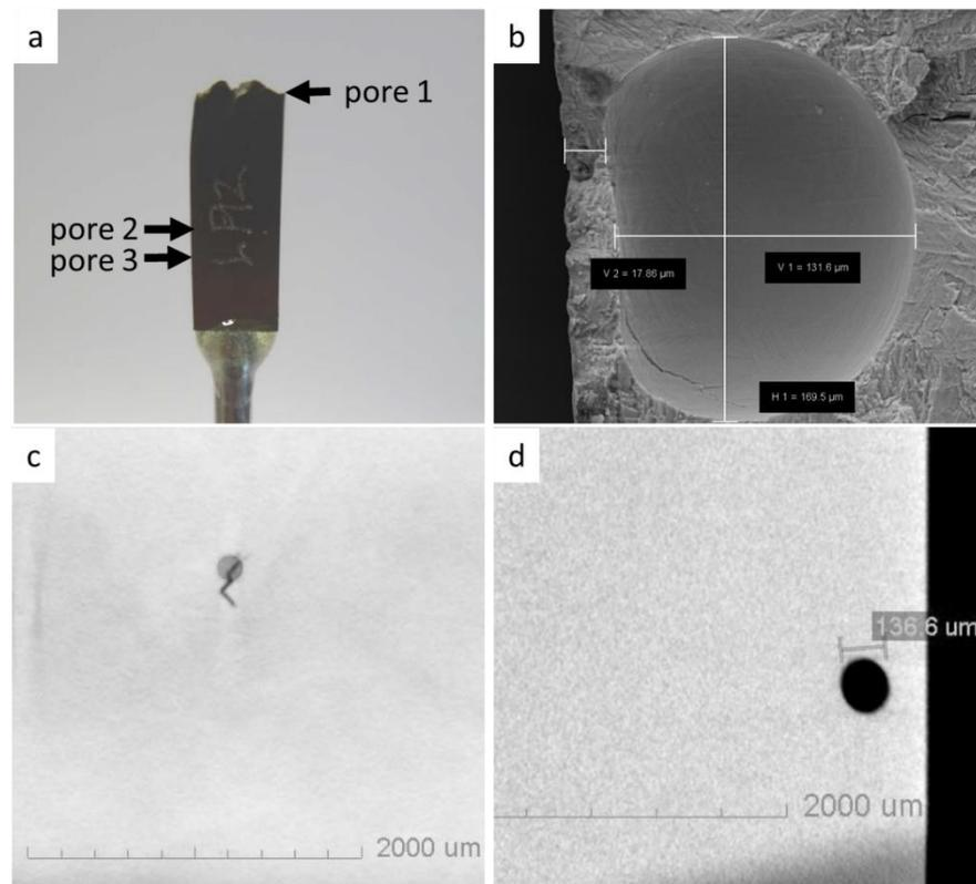
**Figure 11.** TIG welded LCF specimen investigated with XRM: (a) overview of the fractured LCF specimen; (b) SEM fractograph of pore 1, which initiated the fatigue crack that led to failure of the TIG welded LCF specimen; (c) XRM virtual slice of the surface-breaking pore 2, with a diameter of 136  $\mu\text{m}$ , which initiated a 300–400  $\mu\text{m}$  long microcrack; and (d) XRM virtual slice of pore 3 which did not initiate a crack.
