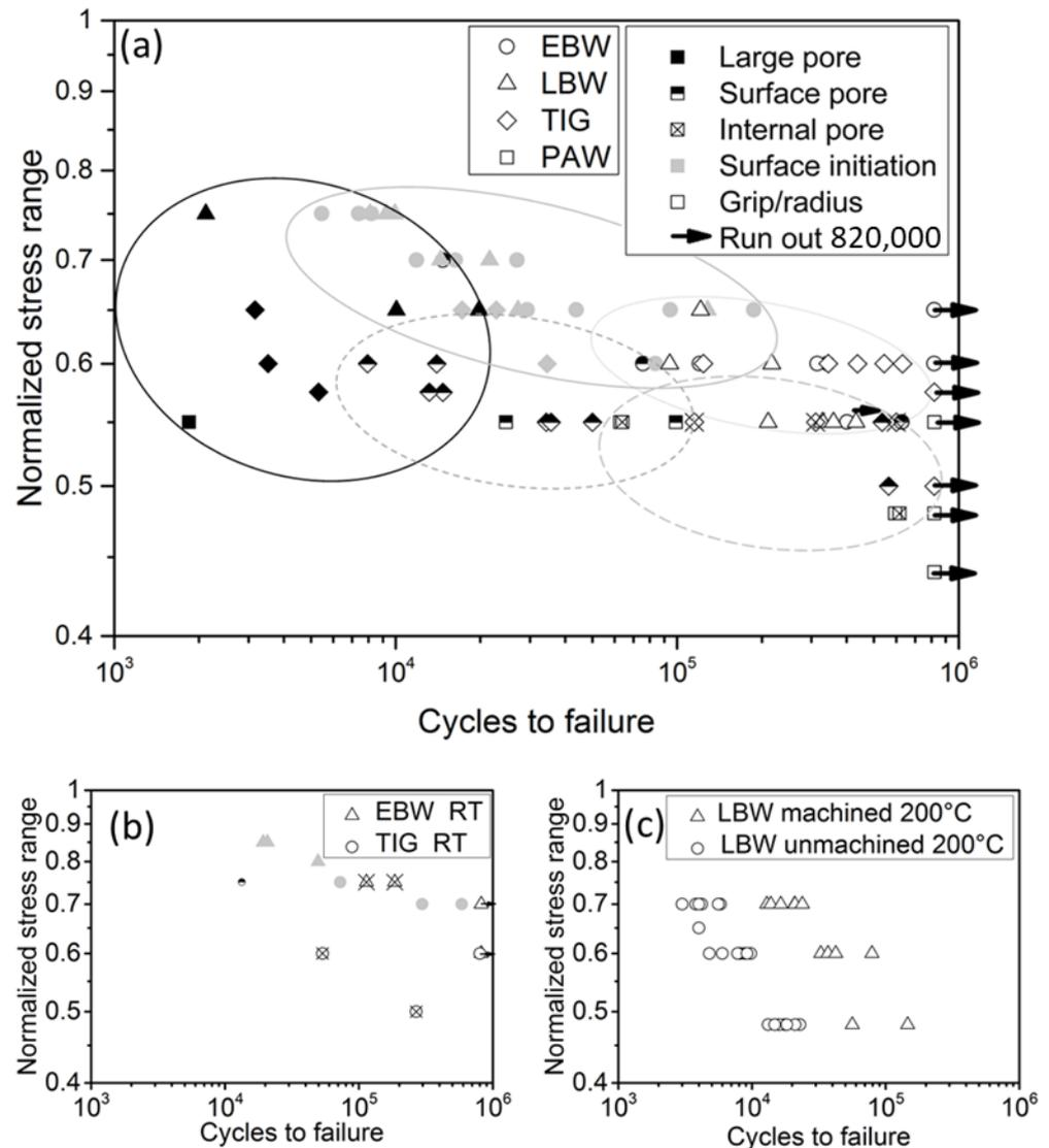
**Figure 7.** LCF results (a) for welds produced by TIG, PAW, EBW, and LBW at 250 °C; (b) EBW and TIG at room temperature; and (c) the effect of weld geometry in LBW. In (a,b), the shape of the symbol indicates the welding process, and the fill of the symbol indicates the type of initiation.
