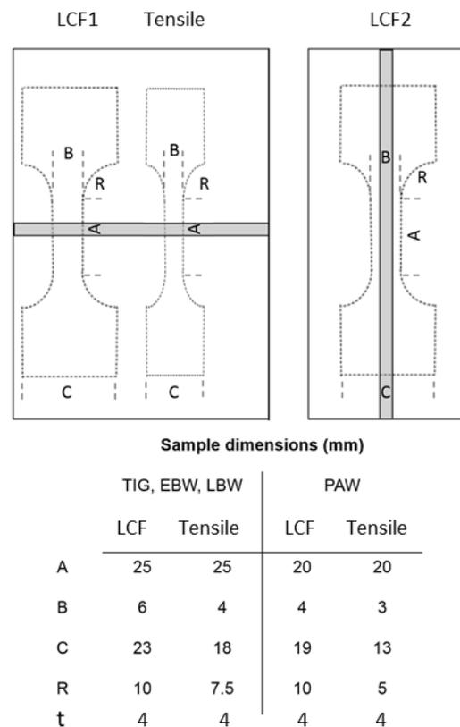
**Figure 1.** Schematic drawings and dimensions of the samples used for mechanical testing. Tensile and LCF type 1 specimens were perpendicular to the weld zone, and the LCF type 2 specimen was parallel to the weld zone.
