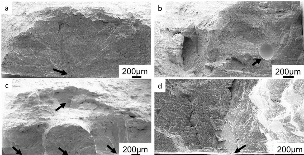
**Figure 9.** Fatigue fracture surfaces showing different types of crack initiation sites: (a) a small pore close to surface (EBW); (b) a large internal pore (TIG); (c) initiations at surface and at a cluster of pores (LBW); and (d) a surface initiation site with a facet (EBW).
