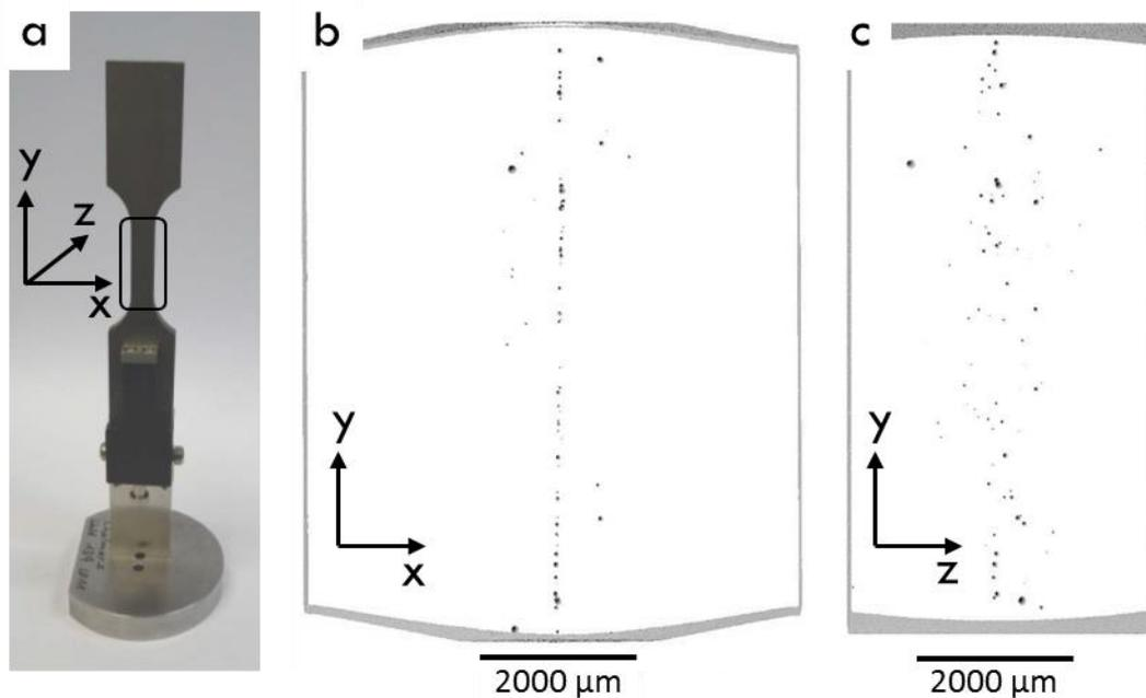
**Figure 12.** XRM 3D volume rendering showing distribution of porosity in a fatigue tested, but not fractured, LCF specimen produced by LBW: (a) overview of the LCF specimen, (b) view from top of the weld, x-y-plane, and (c) view from the side of the weld, y-z-plane.
