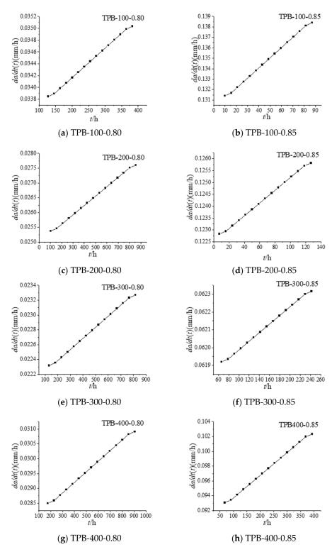
**Figure 2.** Time-dependent fracture curves da/dt (t)-t.
