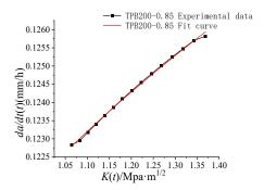
**Figure 3.** Time-dependent fracture curves da/dt (t)-K(t).
