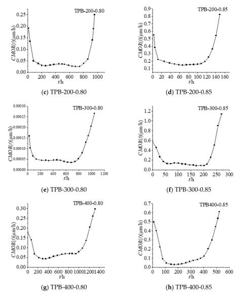
**Figure 1.** Time-dependent fracture curves CMOR(t)-t.
