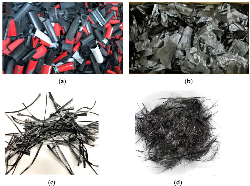
**Figure 4.** The procedure of carbon fiber recycling. (a) CFRP bicycle frame scrap before microwave-assisted pyrolysis; (b) microwave-assisted pyrolysis applied specimen; (c) recycled carbon fiber by cutting; (d) recycled carbon fiber dispersed by pneumatic dispersion.
