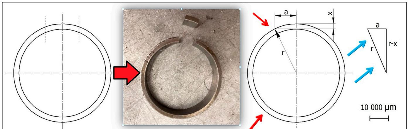
**Figure 2.** Methodology of the angled micro-section used for microhardness measurements (where:  $r$ —radius of the ringed sample,  $a$ —distance from the edge of the angled micro-section,  $x$ —distance from the edge of the perpendicular micro-section).
