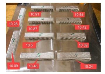
Figure 7. Placement of the test specimens on the build plate and their deformations.
