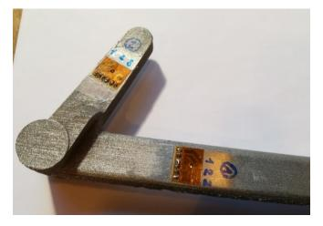
**Figure 2.** Attached strain gauges on the braking pedal at the selected measurement locations. Measurement point (1) and (2) can be observed with drilled holes from HDM.
