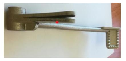
deformation. Figure 3 illustrates the deformation of the braking pedal caused by RS after making a cut at measurement location No. 2 (57.5 mm).
