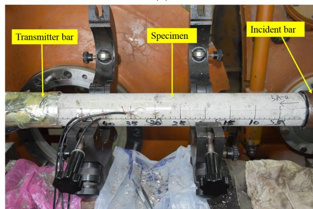
**Figure 3.** Setup of modified Hopkinson bar: (a) schematic diagram of the equipment; (b) photo of the equipment; (c) specimen arrangement.
