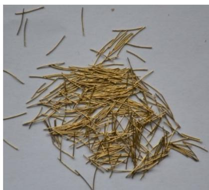
**Figure 1.** Steel fibers used in this study.
