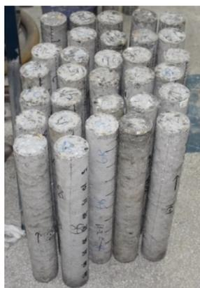
**Figure 2.** Part of the SFRSCC specimens.
