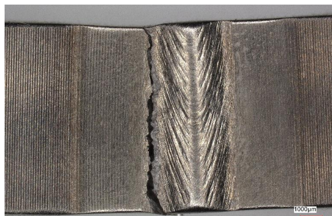
Figure 13. View of the sample (Variant No. II) after the tensile test from the weld face.
