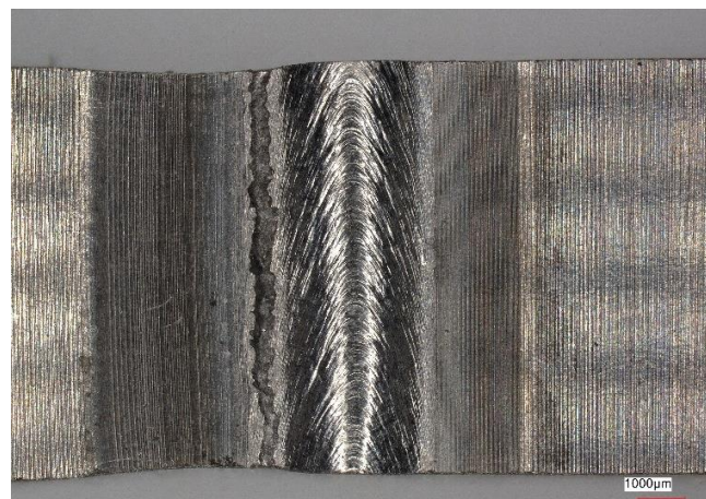
Figure 11. View of the sample (Variant No. I) after the tensile test from the weld face.
