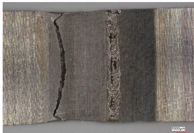
Figure 12. View of the sample (Variant No. I) after the tensile test from the side of the weld ridge.
