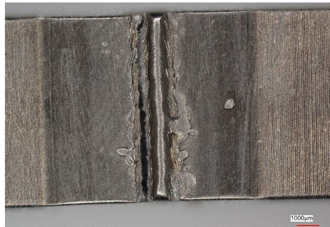
Figure 14. View of the sample (Variant No. II) after the tensile test from the side of the weld ridge.
